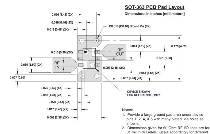
board thicknesses and dielectric contants.We recommend 1 or 2 ounce copper. Measurements for this data sheet were made on a 31 mil thick Getek with 1 ounce copper on both sides.
