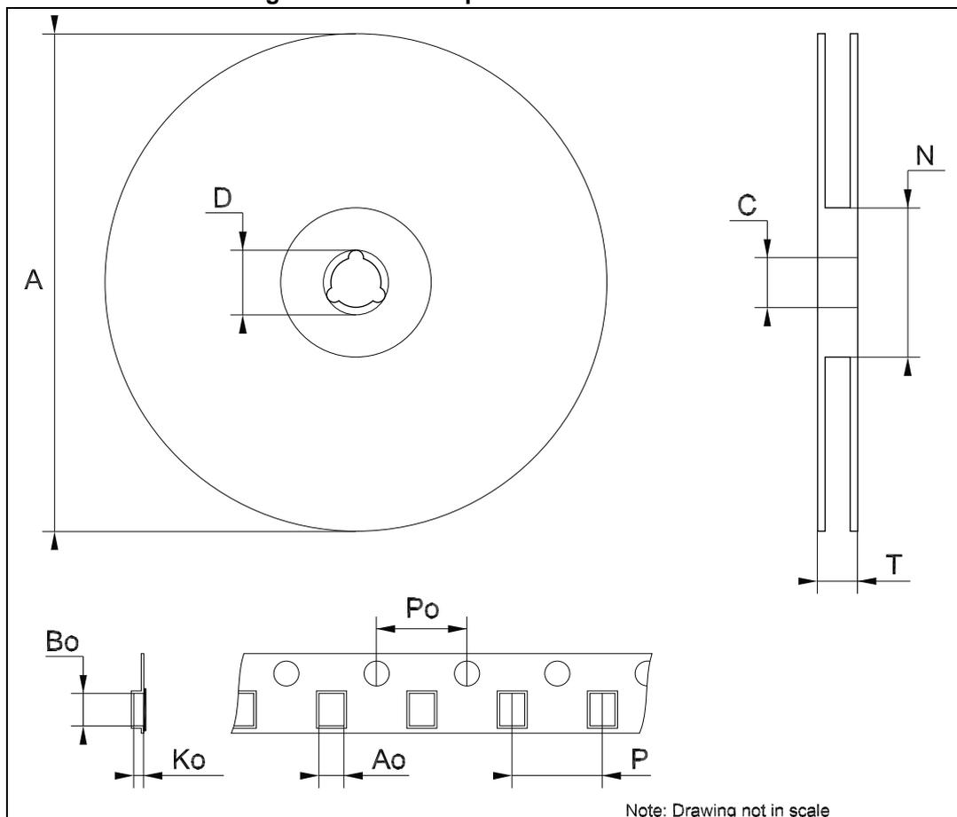
Table 6. P<sup>2</sup>PAK tape and reel mechanical data
