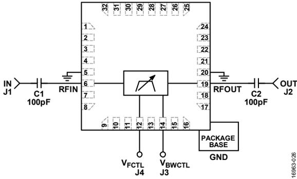
Figure 26. Typical Application Circuit
