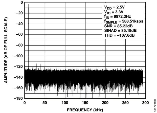
Figure 20. 10 kHz FFT,  $V_{REF} = 2.5V$
