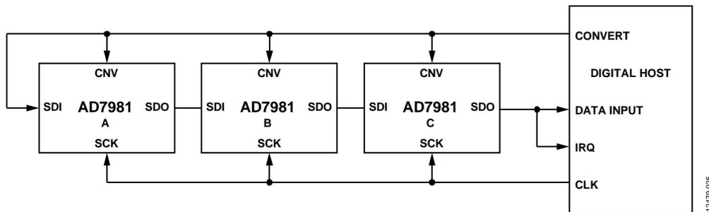
Figure 51. Chain Mode with Busy Indicator Connection Diagram
