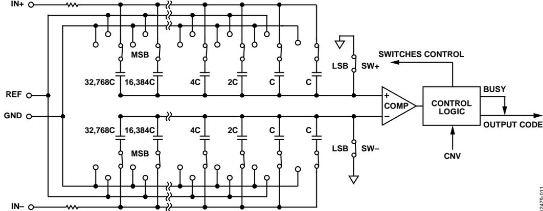
Figure 35. ADC Simplified Schematic
