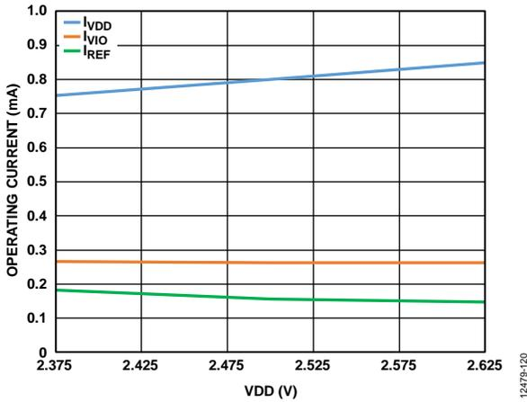
Figure 31. Operating Current vs. Supply Voltage (VDD)
