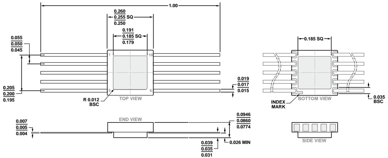
Figure 57. 10-Lead Ceramic Flat Package [FLATPACK] (F-10-2)
