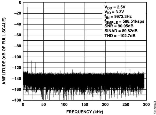
Figure 17. 10 kHz FFT,  $V_{REF} = 5.0V$
