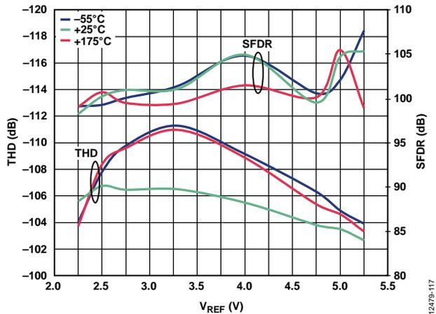
Figure 19. THD and SFDR vs. Reference Voltage ( $V_{REF}$ ), MSOP
