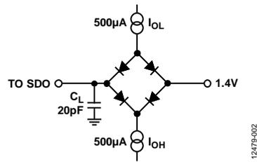
Figure 2. Load Circuit for Digital Interface Timing
