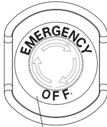
"EMERGENCY STOP" is indicated on A22Z-EG1-W. Legend plate is not provided with A22Z-EG10 and A22Z-EG10-W.
