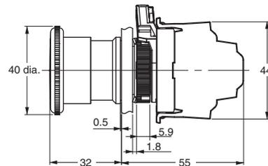
**Note:** Unless otherwise specified, a tolerance of  $\pm 0.8\text{mm}$  applies to all dimensions.
