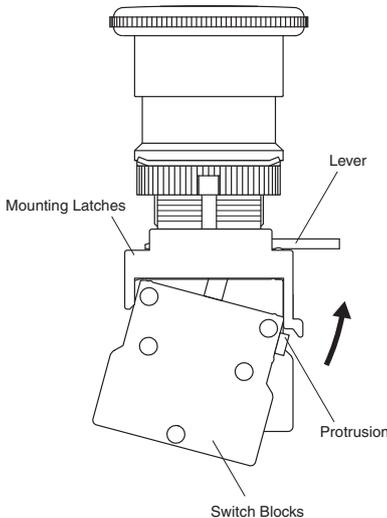
(2) Removing the Switch Blocks
