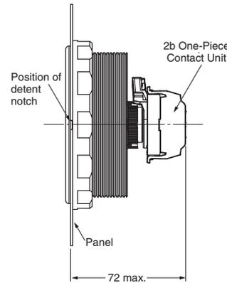
**Push-in Plus Terminal Block Type Mounting a 2-pole Switch Unit \***
