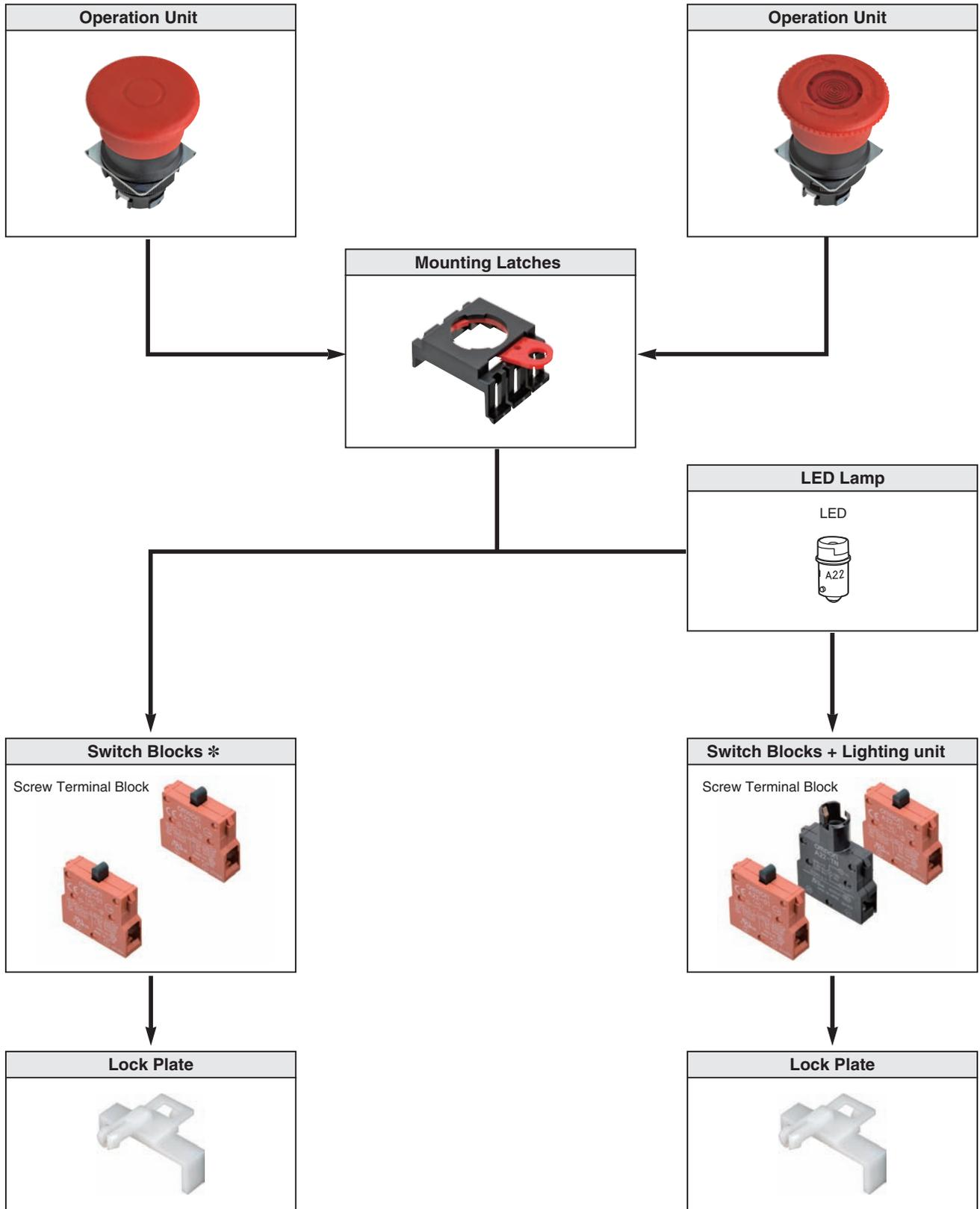
\* Up to three Switch Blocks can be mounted for multiple contacts.
