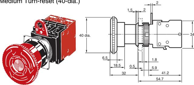
Switch dimensions when mounted to a 2NO (2NC) one-piece switch block
