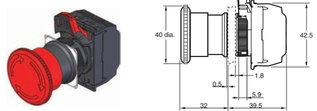
**Note:** The dimensions the same even if the Operation Unit is replaced with the A22NE-MR□-N or the A22NE-MR□-N-RD.
