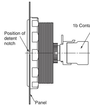
**Screw Terminal Block Type Mounting a 2-pole Switch Unit \***
