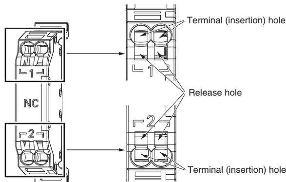
**Connecting Wires with Ferrules and Solid Wires**
