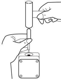
(3) Securing the Connector Cable
