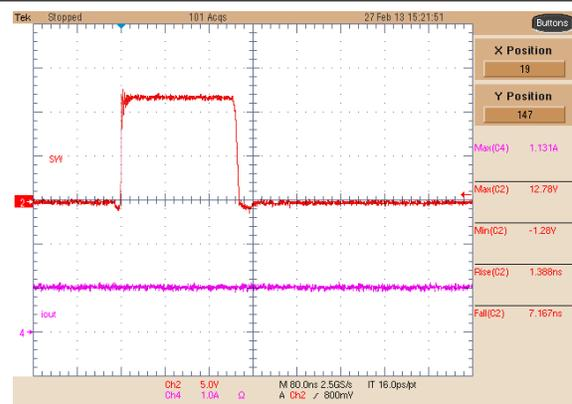
**Figure 8-8. Buck 1 Switching Node, 1-A Load**
