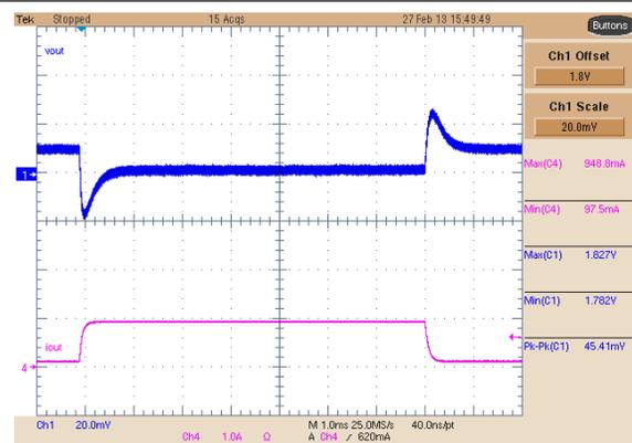
**Figure 8-28. Buck 2 Dynamic Response, 0-A to 1-A Step**
