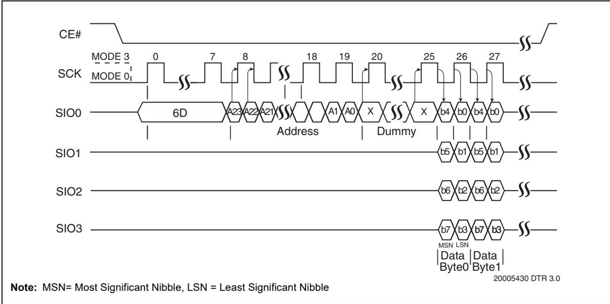
FIGURE 5-18: SPI QUAD OUTPUT READ – DTR
