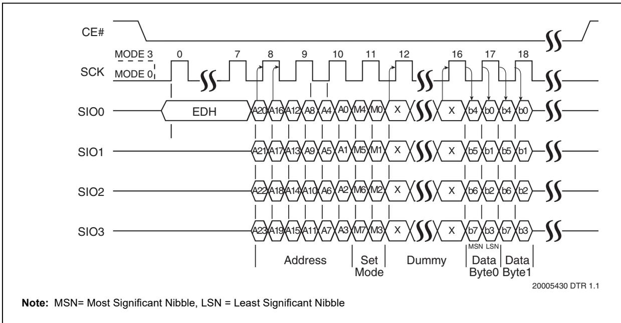
FIGURE 5-16: SPI QUAD I/O READ – DTR
