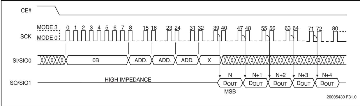
In SQI protocol, the host drives CE# low then sends the Read command cycle command, 0BH, followed by three address cycles, a Set Mode Configuration cycle, and two dummy cycles. Each cycle is two nibbles (clocks) long, most significant nibble first.
