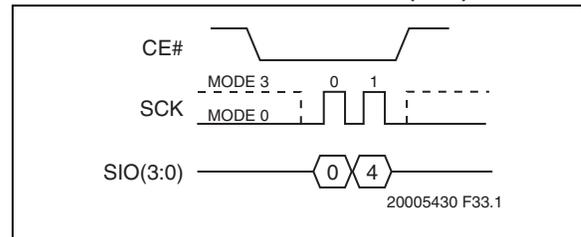
**FIGURE 5-41: WRITE-DISABLE (WRDI) SEQUENCE (SPI)**
