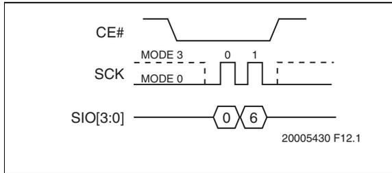
**FIGURE 5-39: WRITE-ENABLE SEQUENCE (SPI)**
