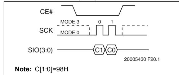
**FIGURE 5-51: GLOBAL BLOCK-PROTECTION UNLOCK (SPI)**
