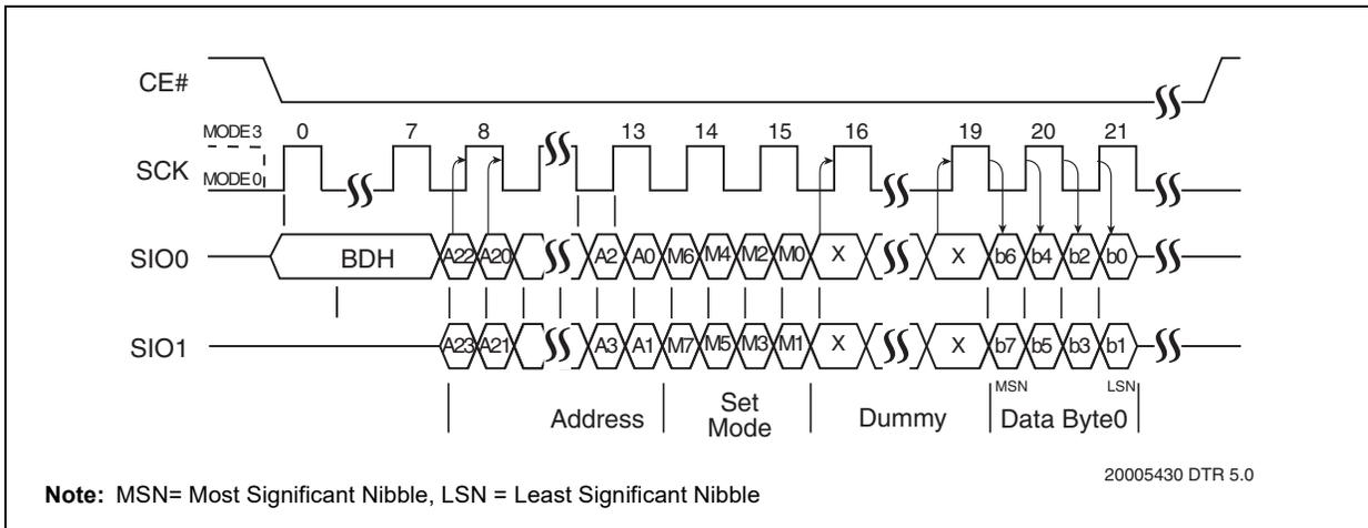
FIGURE 5-20: SPI DUAL I/O READ – DTR
