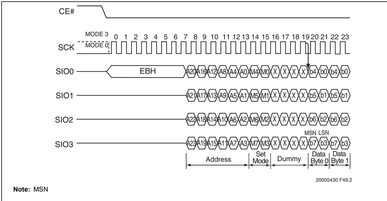
FIGURE 5-10: BACK-TO-BACK SPI QUAD I/O READ SEQUENCES WHEN M[7:0] = AXH
