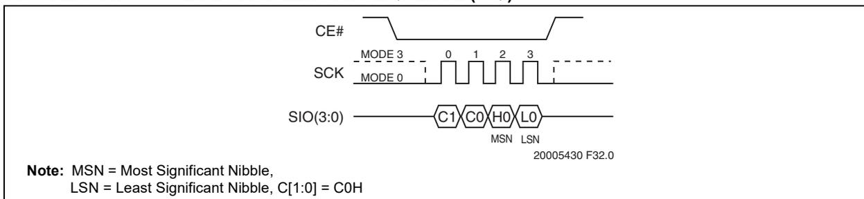
FIGURE 5-12: SET BURST LENGTH SEQUENCE (SPI)
