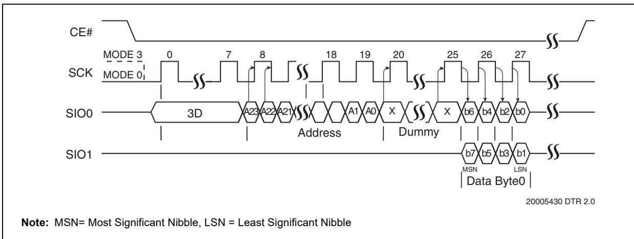
FIGURE 5-17: SPI DUAL OUTPUT READ – DTR
