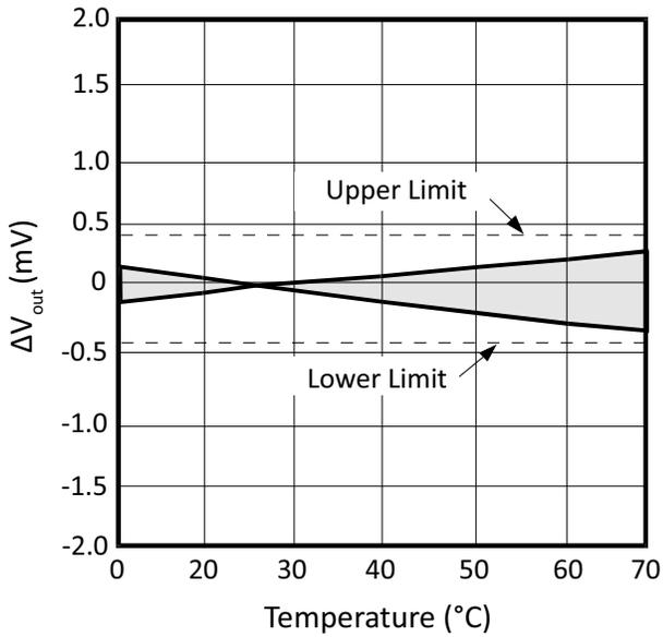
Figure 3:  $V_{OUT}$  vs. Temperature (VRE310J)
