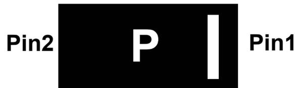
Note: The marking can be rotated by multiples of 90° to differentiate assemble location. In no case should this product marking be used to orient the component for its placement on a PCB. Only pin 1 mark is to be used for this purpose.
