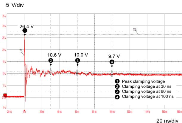
**Figure 7. ESD response to IEC 61000-4-2 (-8kV contact discharge)**
