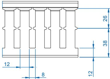
3x4, 4x4 and 6x4" duct does not have middle mounting row of slots
