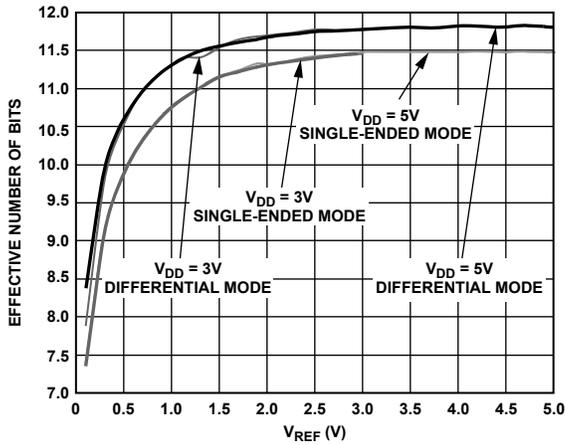
Figure 11. Effective Number of Bits vs.  $V_{REF}$
