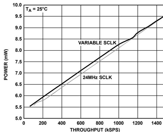
Figure 39. Power vs. Throughput in Normal Mode with  $V_{DD} = 3$  V
