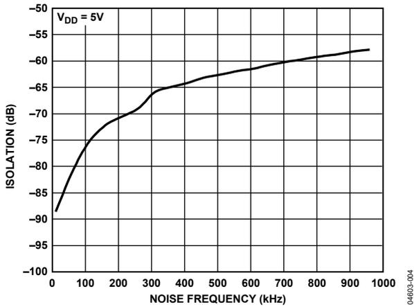
Figure 5. Channel-to-Channel Isolation
