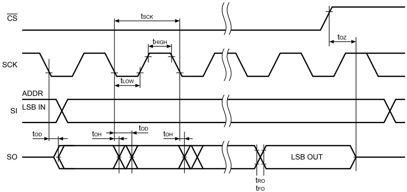
Figure 8 Serial Output Timing
