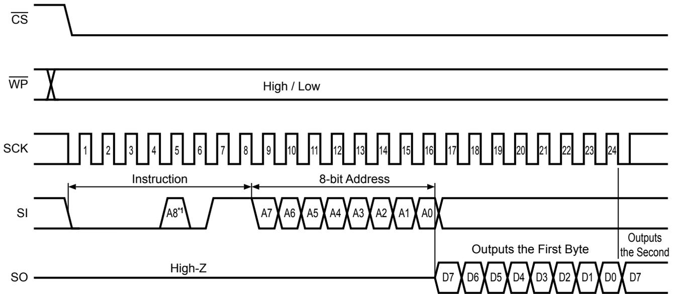
\*1 In the S-25C040A, assign bit A8 in the address into the fifth bit in an instruction code.
