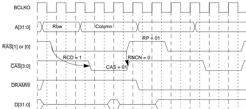
Figure 11-6. Basic Non-Page-Mode Operation RCD = 1, RNCN = 0 (5-5-5)
