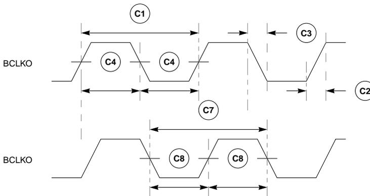
Note: Input and output AC timing specifications are measured to BCLKO with a 50-pF load capacitance (not including pin capacitance).
