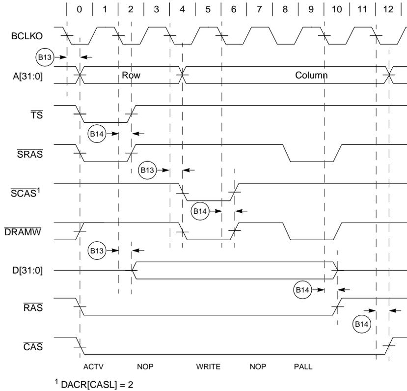
**Figure 20-9. SDRAM Write Cycle with EDGESEL Tied Low**
