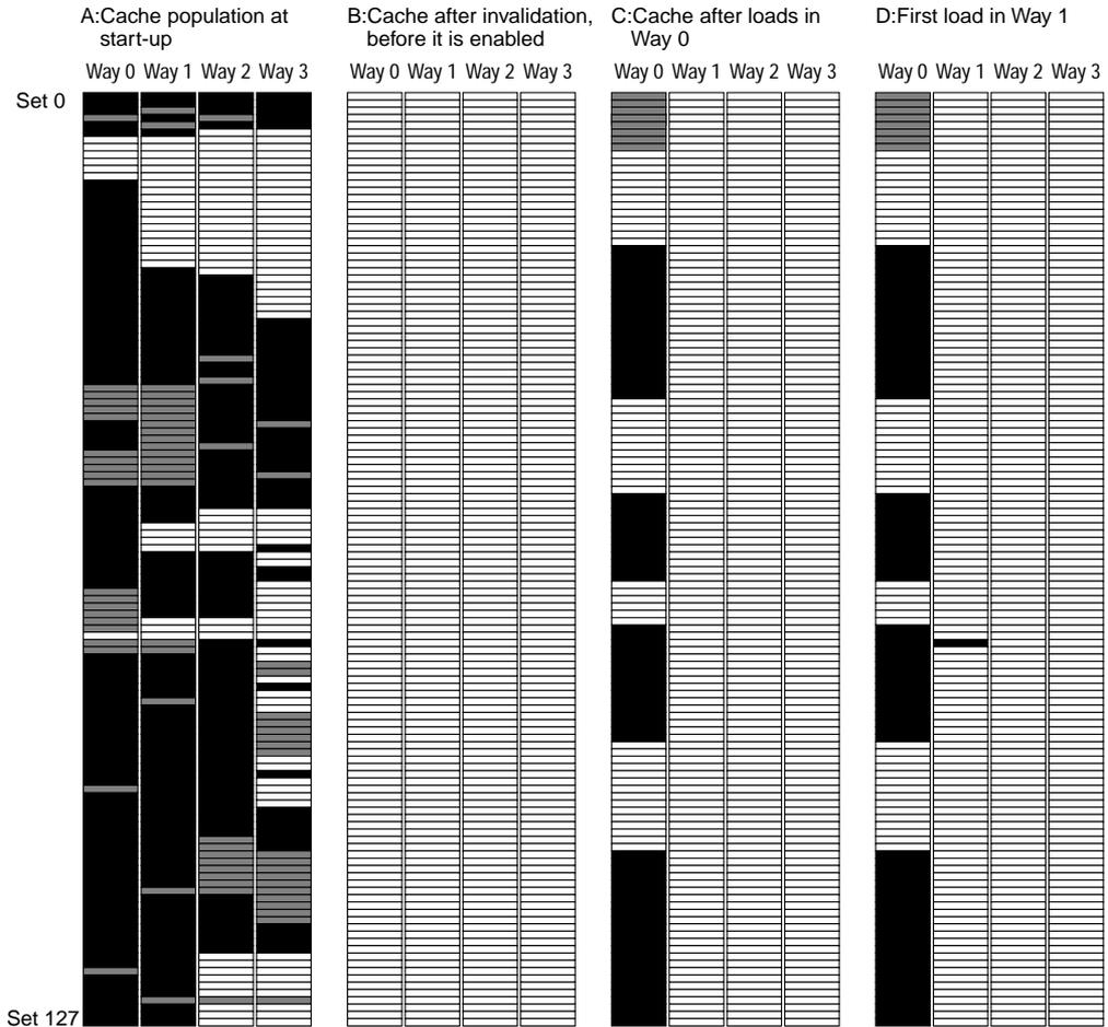
At reset, cache contents are indeterminate; V and M may be set. The cache should be cleared explicitly by setting CACR[CINVA] before the cache is enabled.
