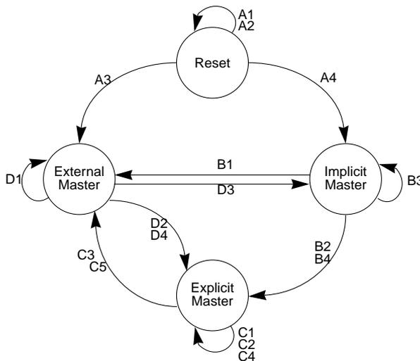
**Figure 18-29. MCF5307 Two-Wire Bus Arbitration Protocol State Diagram**
