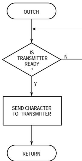
**Figure 14-27. UART Mode Programming Flowchart (Sheet 5 of 5)**
