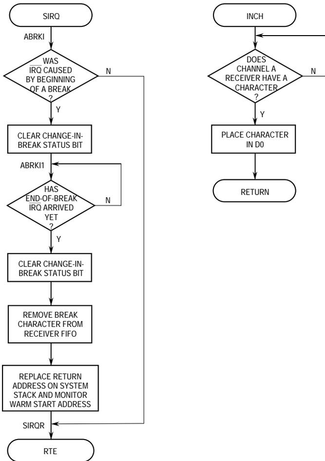
Figure 14-27. UART Mode Programming Flowchart (Sheet 4 of 5)
