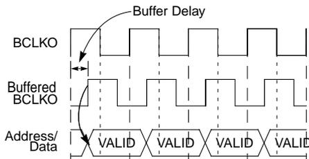
**Figure 11-14. Using EDGESEL to Change Signal Timing**
