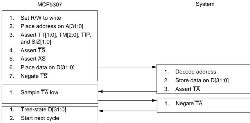
**Figure 18-7. Write Cycle Flowchart**
