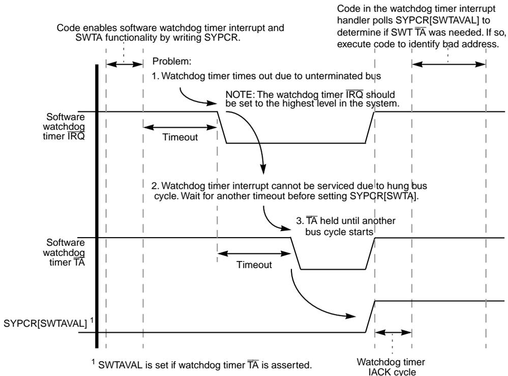
**Figure 6-4. MCF5307 Embedded System Recovery from Unterminated Access**
