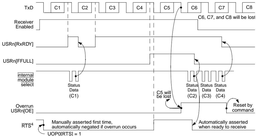
Figure 14-22. Receiver Timing
