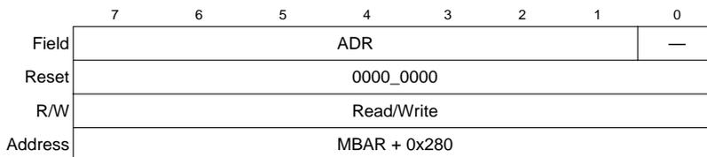
**Figure 8-5. I<sup>2</sup>C Address Register (IADR)**
