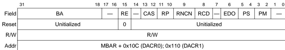
**Figure 11-3. DRAM Address and Control Registers (DACR0/DACR1)**
