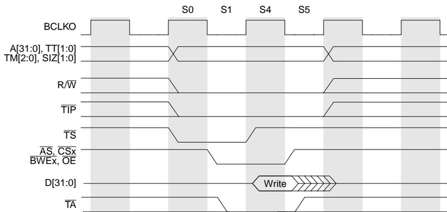
**Figure 18-10. Write Cycle with Fast Termination**
