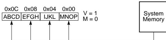
3. After the cache line is filled, the write that initiated the write miss (the character X) completes to 0x0B.
