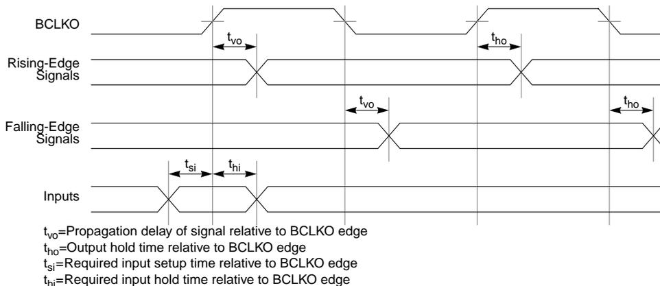
Figure 18-1. Signal Relationship to BCLKO for Non-DRAM Access
