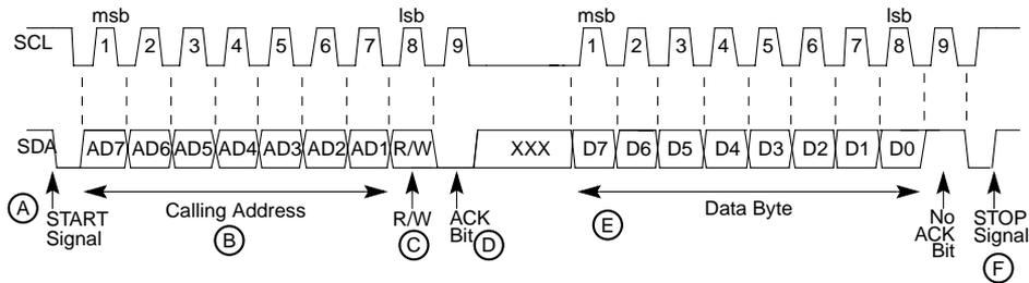
**Figure 8-2. I<sup>2</sup>C Standard Communication Protocol**
