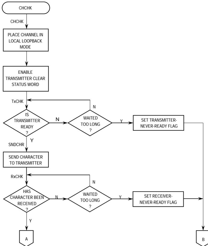
Figure 14-27. UART Mode Programming Flowchart (Sheet 2 of 5)
