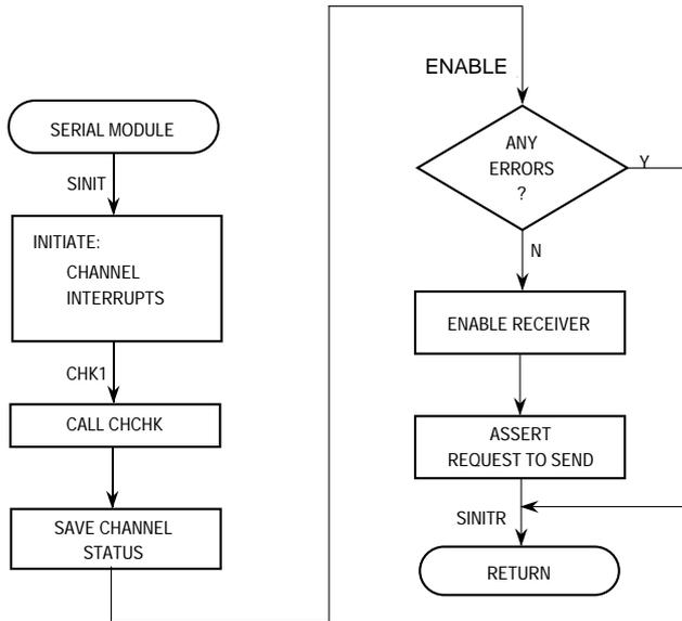
**Figure 14-27. UART Mode Programming Flowchart (Sheet 1 of 5)**
