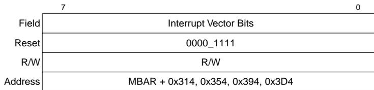
**Figure 12-10. DMA Interrupt Vector Registers (DIVR<sub>n</sub>)**
