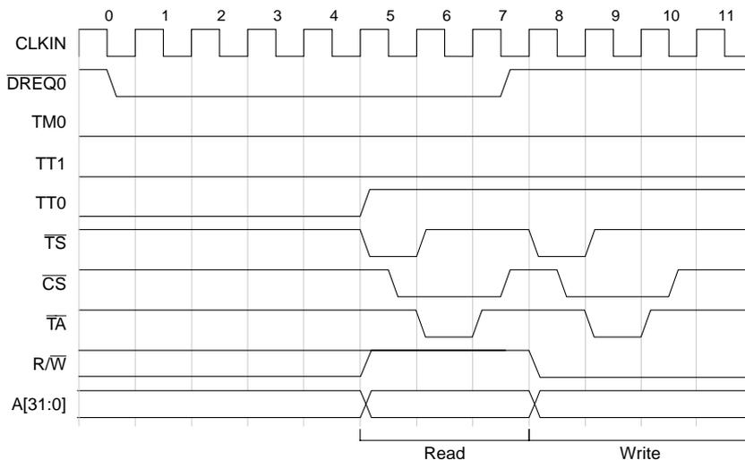
**Figure 12-11.  $\overline{\text{DREQ}}$  Timing Constraints, Dual-Address DMA Transfer**
