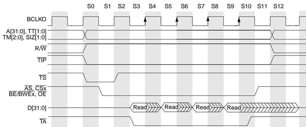
Figure 18-19. Longword Read from an 8-Bit Port, External Termination
