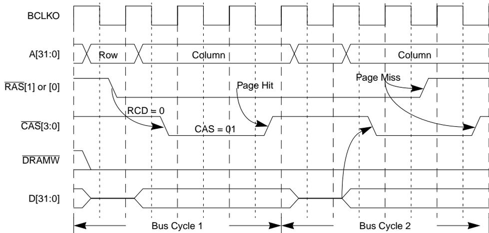
Figure 11-10. Write Hit in Continuous Page Mode
