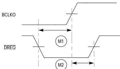
**Figure 20-18. DMA Timing**
