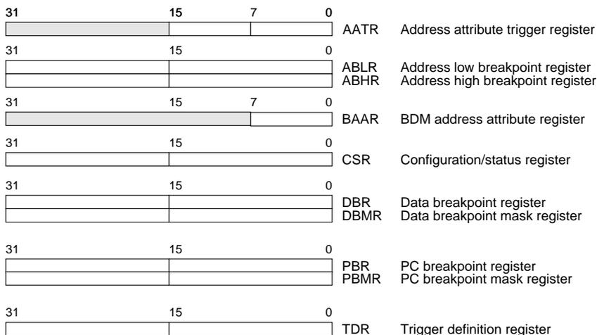
Note: Each debug register is accessed as a 32-bit register; shaded fields above are not used (don't care). All debug control registers are writable from the external development system or the CPU via the WDEBBUG instruction. CSR is write-only from the programming model. It can be read or written through the BDM port using the RDMREG and WDMREG commands.
