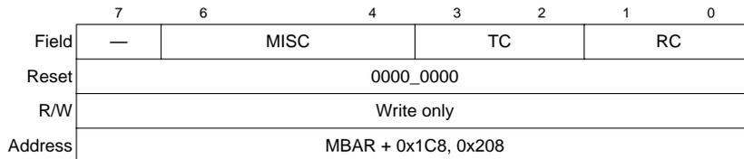
**Figure 14-6. UART Command Register (UCR $n$ )**
