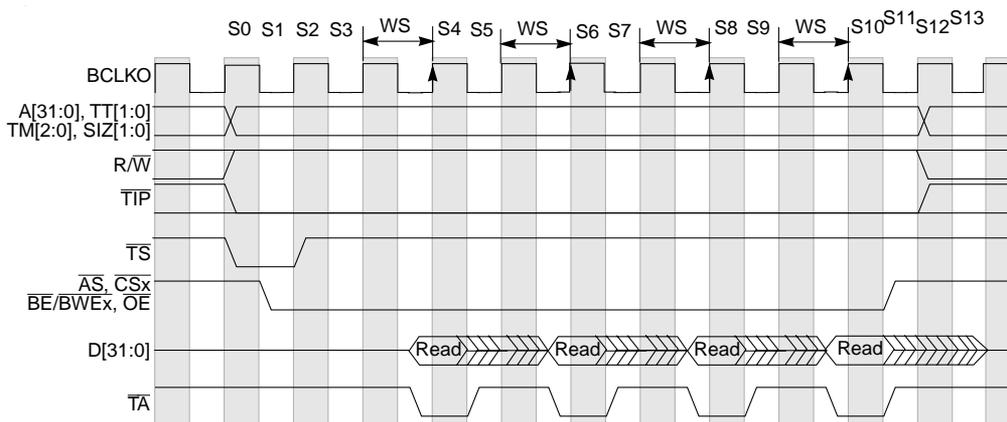
Figure 18-14. Line Read Burst (3-2-2-2), External Termination
