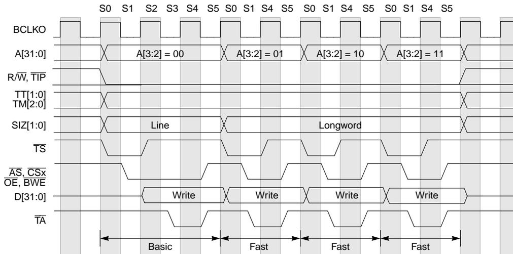
**Figure 18-18. Line Write Burst-Inhibited, Internal Termination**
