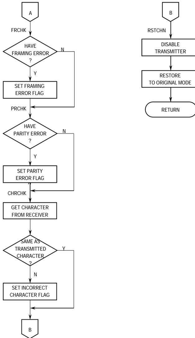
**Figure 14-27. UART Mode Programming Flowchart (Sheet 3 of 5)**
