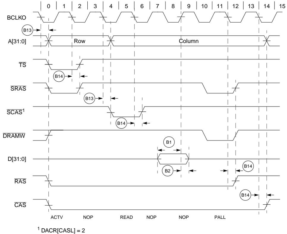
**Figure 20-8. SDRAM Read Cycle with EDGESEL Tied Low**
