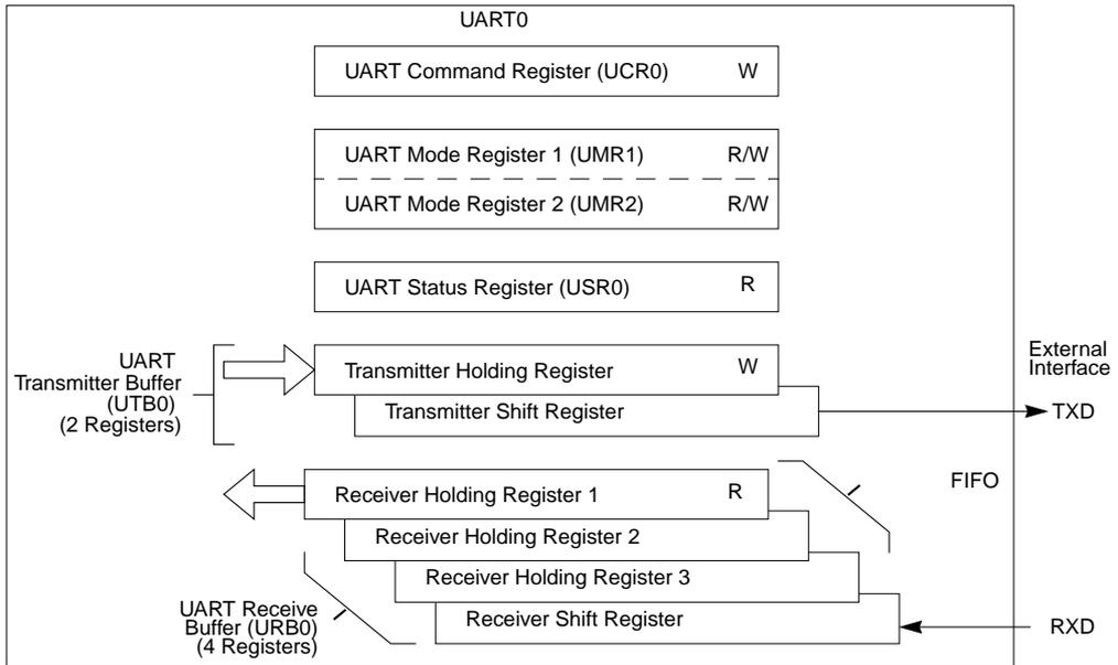
**Figure 14-20. Transmitter and Receiver Functional Diagram**
