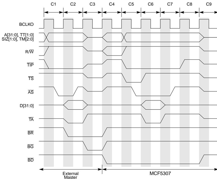
**Figure 18-31. Three-Wire Bus Arbitration**
