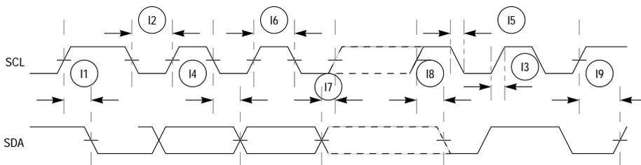
**Figure 20-15. I<sup>2</sup>C Input/Output Timings**
