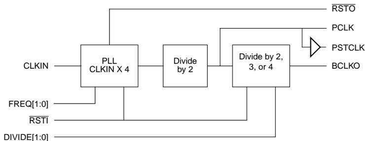
Figure 7-1. PLL Module Block Diagram
