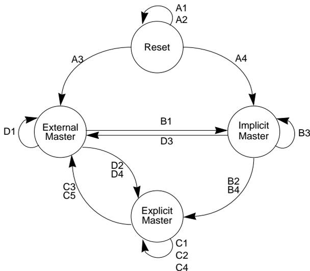
**Figure 18-32. Three-Wire Bus Arbitration Protocol State Diagram**
