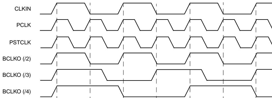
NOTE: The clock signals are shown with edges aligned to show frequency relationships only. Actual signal edges have some skew between them.
