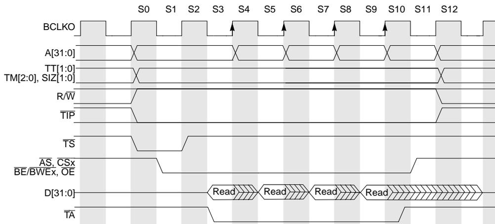
Figure 18-13. Line Read Burst (2-1-1-1), Internal Termination
