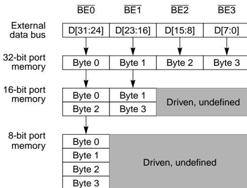
Figure 10-1. Connections for External Memory Port Sizes
