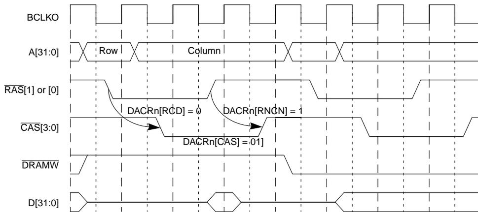
**Figure 11-5. Basic Non-Page-Mode Operation RCD = 0, RNCN = 1 (4-4-4-4)**
