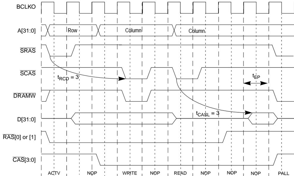
**Figure 11-21. Synchronous, Continuous Page-Mode Access—Read after Write**
