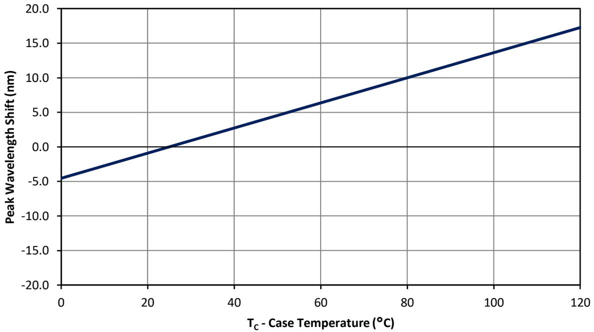
Figure 9: Typical peak wavelength shift vs. case temperature.
