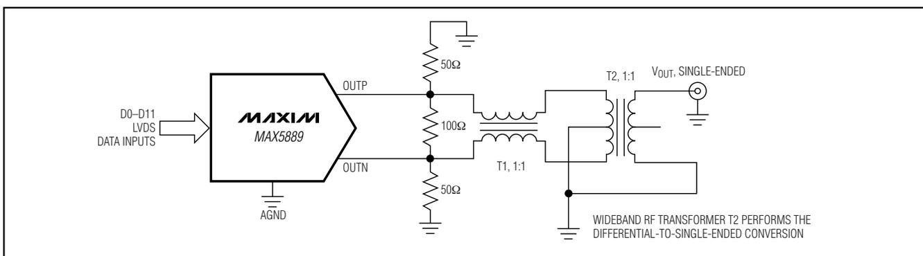
Figure 5. Differential-to-Single-Ended Conversion Using a Wideband RF Transformer
