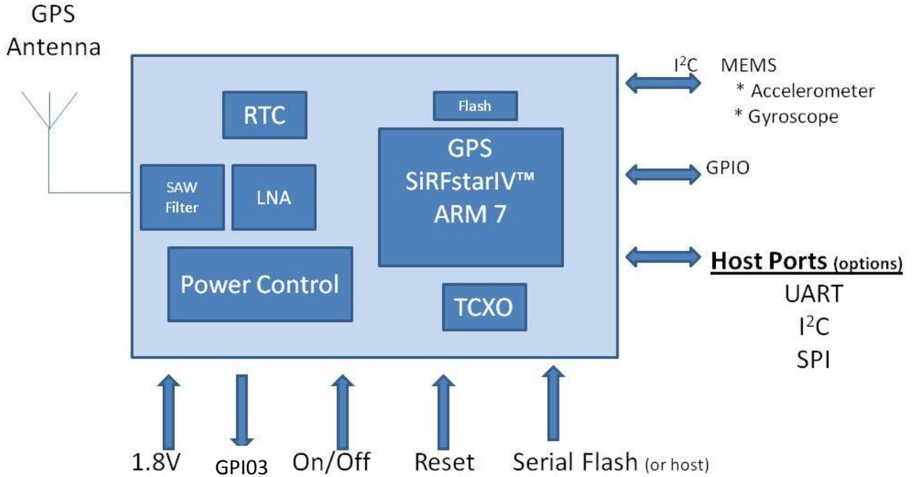
**Figure 1 Inventek's ISM480F1 General Block Diagram**
