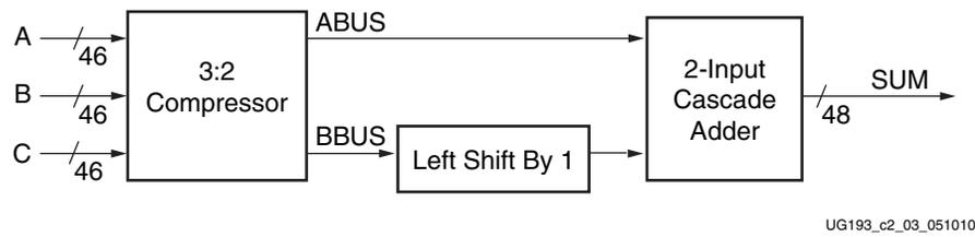
Figure 2-3: Three-Input Adder
