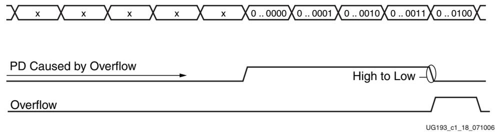
Figure 1-18: Overflow Condition in the Pattern Detector
