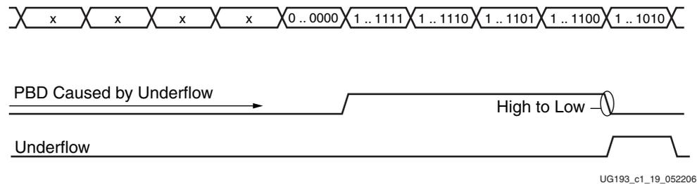
Figure 1-19: Underflow Condition in the Pattern Detector
