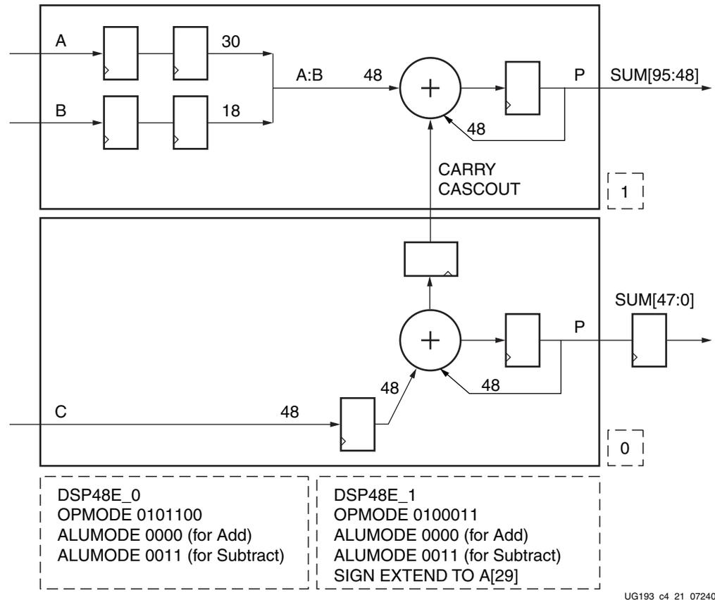
Figure 4-22: 96-Bit Accumulator
