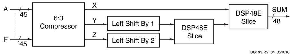
Figure 2-4: Six-Input Adder
