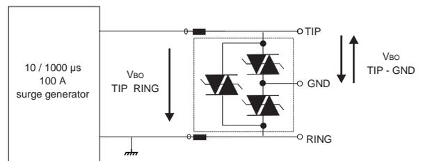
**Fig. 5-1 : Breakover voltage measurement (TLP140M/G/G-1).**
