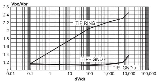
**Fig. 5-3 : Breakover voltage measurement (TLP270M/G/G-1).**
