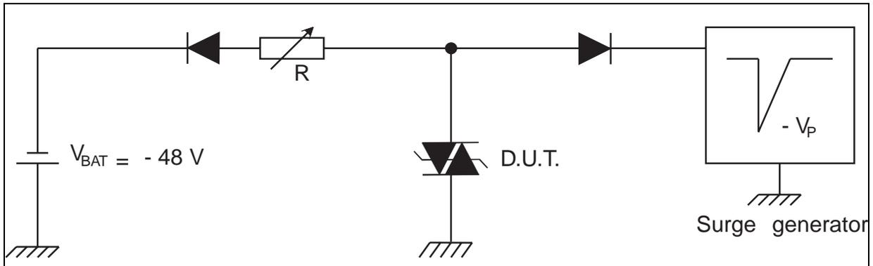
This is a GO-NO GO test which allows to confirm the holding current (I<sub>H</sub>) level in a functional test circuit.
