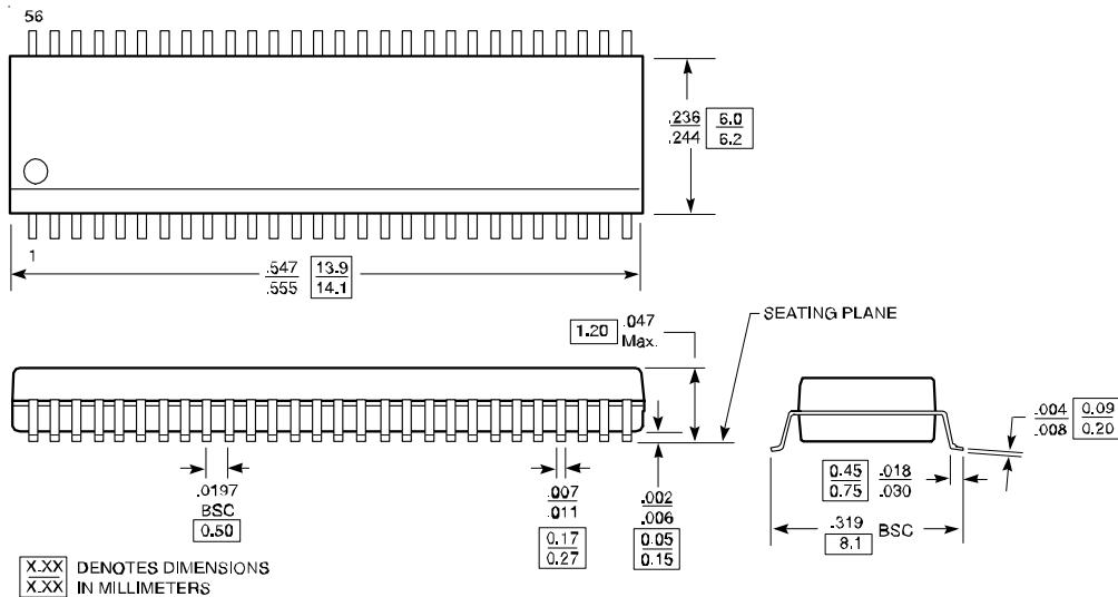
**Packaging Mechanical: 56-Pin SSOP (V)**
