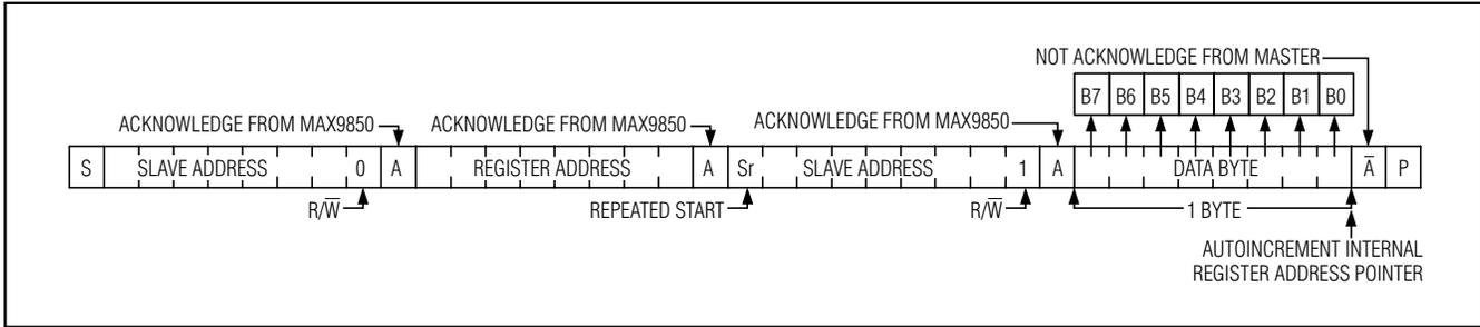
Figure 10. Reading One Byte of Data from MAX9850
