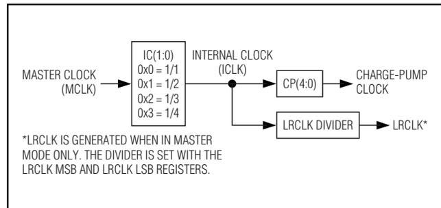
Figure 3. Internally Generated Clock Signals Derived from MCLK
