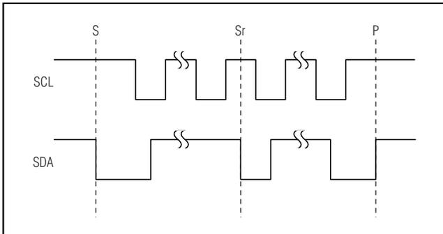
Figure 6. START, STOP, and REPEATED START Conditions
