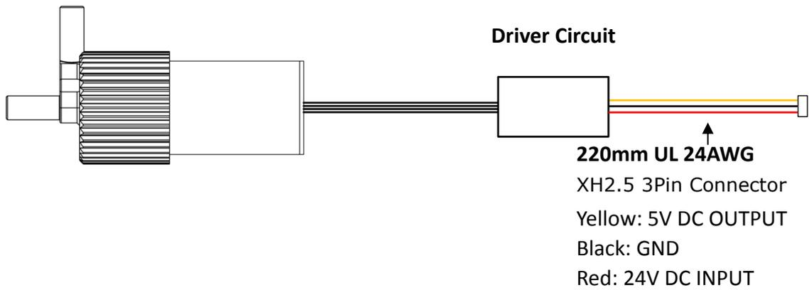
Fig. 1 Wire Schematic
