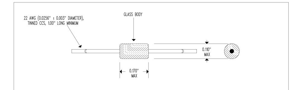
RESISTANCE @  $+25^{\circ}C = 100 \Omega \pm 10\%$ RESISTANCE TEMPERATURE CURVE = "B"
