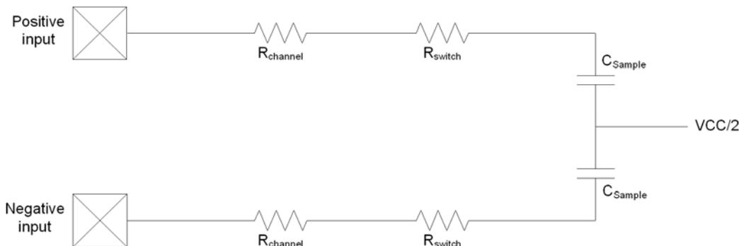
In order to achieve  $n$  bits of accuracy, the source output resistance,  $R_{source}$ , must be less than the ADC input resistance on a pin:
