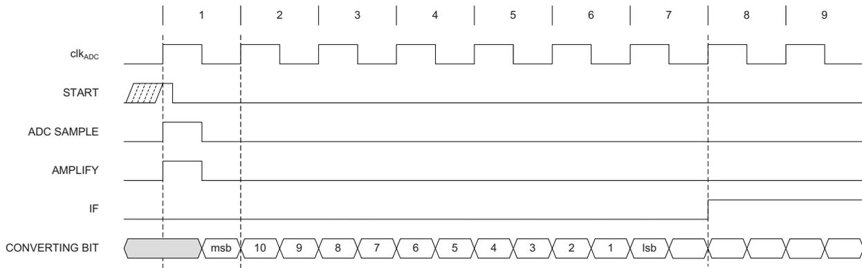
**Figure 26-16. ADC timing for one single conversion with 8x gain.**
