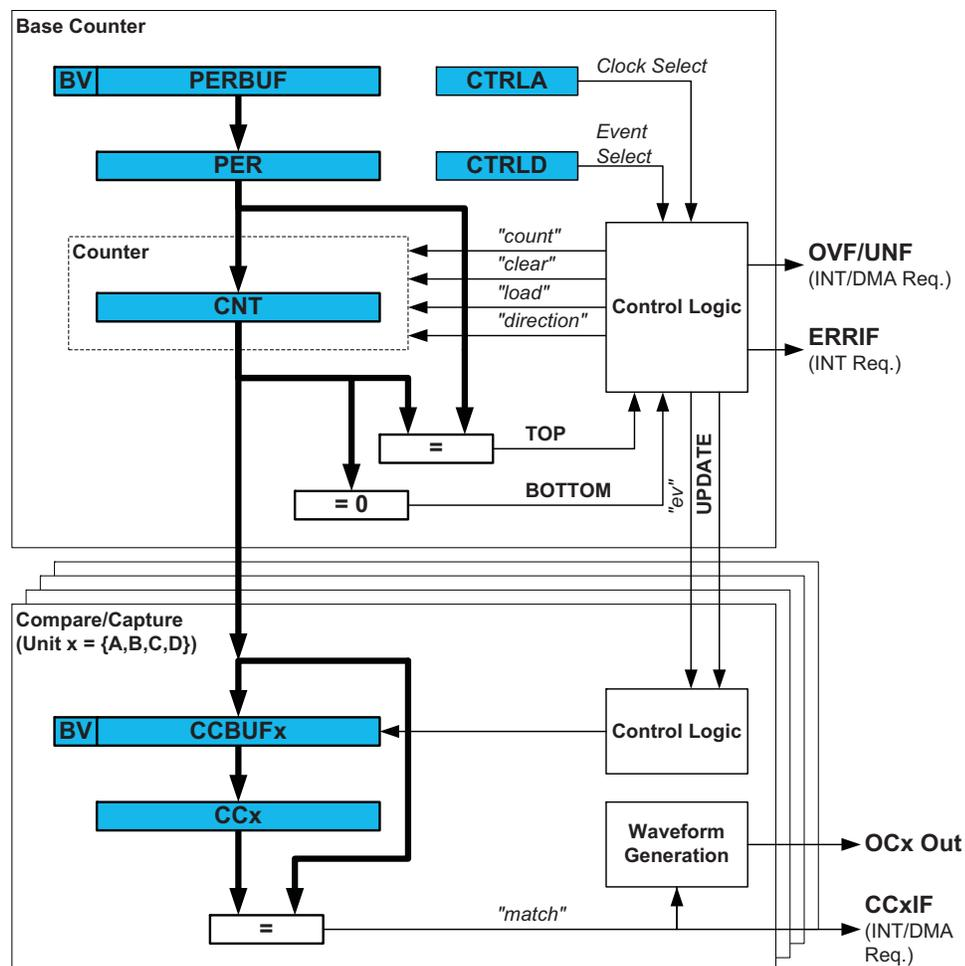
The counter register (CNT), period registers with buffer (PER and PERBUF), and compare and capture registers with buffers (CCx and CCxBUF) are 16-bit registers. All buffer register have a buffer valid (BV) flag that indicates when the buffer contains a new value.
