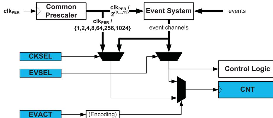
The peripheral clock is fed into a common prescaler (common for all timer/counters in a device). Prescaler outputs from 1 to  $1/1024$  are directly available for selection by the timer/counter. In addition, the whole range of prescaling from 1 to  $2^{15}$  times is available through the event system.
