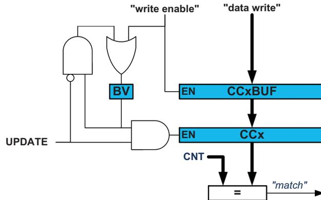
When the CC channels are used for a capture operation, a similar double buffering mechanism is used, but in this case the buffer valid flag is set on the capture event, as shown in Figure 13-5. For capture, the buffer register and the corresponding CCx register act like a FIFO. When the CC register is empty or read, any content in the buffer register is passed to the CC register. The buffer valid flag is passed to set the CCx interrupt flag (IF) and generate the optional interrupt.
