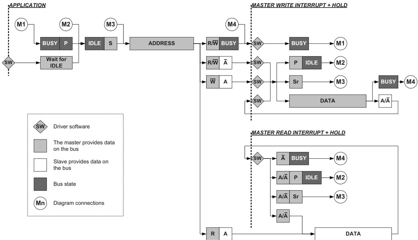
The number of interrupts generated is kept to a minimum by automatic handling of most conditions. Quick command and smart mode can be enabled to auto-trigger operations and reduce software complexity.
