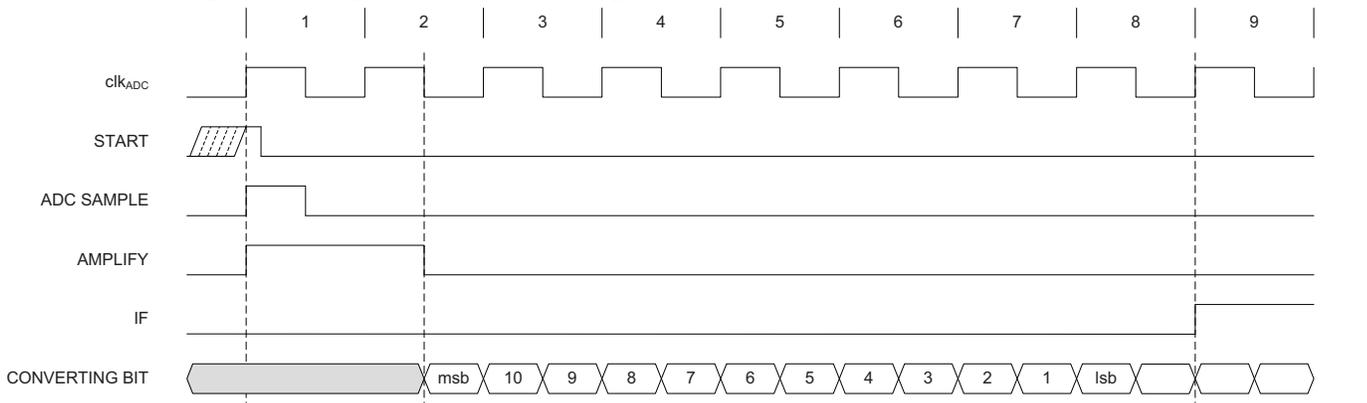
Figure 26-17. ADC timing for one single conversion with 64x gain.
