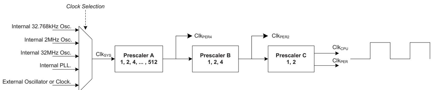
Prescaler A divides the system clock, and the resulting clock is clk<sub>PER4</sub>. Prescalers B and C can be enabled to divide the clock speed further to enable peripheral modules to run at twice or four times the CPU clock frequency. If Prescalers B and C are not used, all the clocks will run at the same frequency as the output from Prescaler A.
