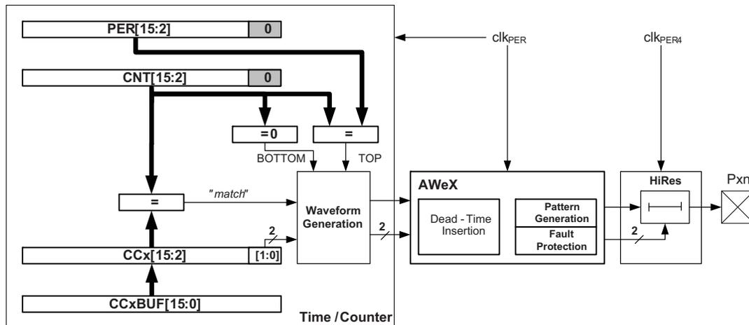
When the hi-res extension is enabled, the timer/counter must run from a non-prescaled peripheral clock. The timer/counter will ignore its two least-significant bits (lsb) in the counter, and counts by four for each peripheral clock cycle. Overflow/underflow and compare match of the 14 most-significant bits (msb) is done in the timer/counter. Count and compare of the two lsb is handled and compared in the hi-res extension running from the peripheral 4x clock.
