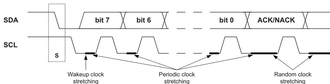
Note: 1. Clock stretching is not supported by all I<sup>2</sup>C slaves and masters.
