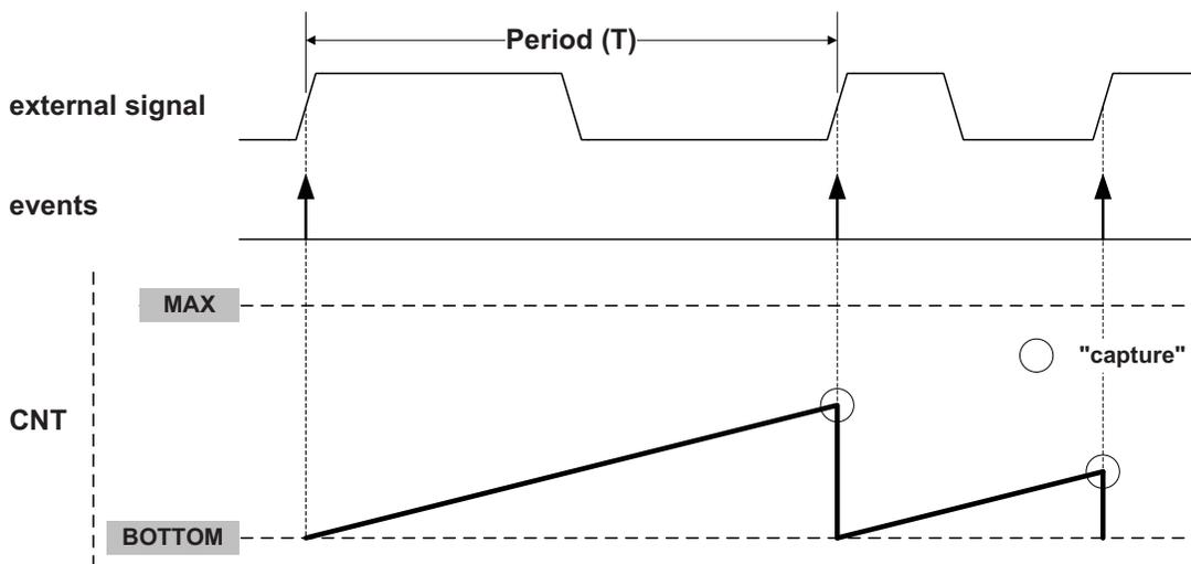
Since all capture channels use the same counter (CNT), only one capture channel must be enabled at a time. If two capture channels are used with different sources, the counter will be restarted on positive edge events from both input sources, and the result will have no meaning.
