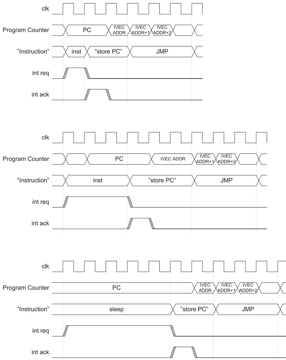
If an interrupt occurs when the device is in sleep mode, the interrupt execution response time is increased by five clock cycles. In addition, the response time is increased by the start-up time from the selected sleep mode.
