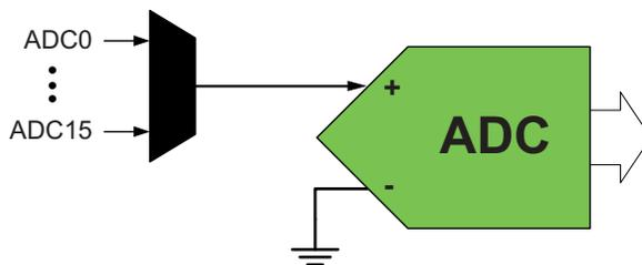
In unsigned mode, the negative input is connected to half of the voltage reference (VREF) voltage minus a fixed offset. The nominal value for the offset is:
