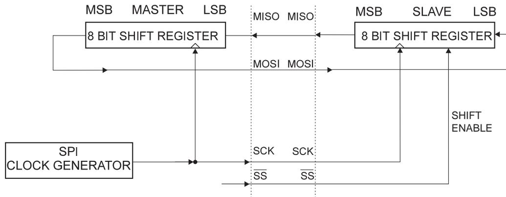
The SPI module is unbuffered in the transmit direction and single buffered in the receive direction. This means that bytes to be transmitted cannot be written to the SPI DATA register before the entire shift cycle is completed. When receiving data, a received character must be read from the DATA register before the next character has been completely shifted in. Otherwise, the first byte will be lost.
