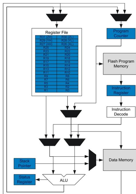
The arithmetic logic unit (ALU) supports arithmetic and logic operations between registers or between a constant and a register. Single-register operations can also be executed in the ALU. After an arithmetic operation, the status register is updated to reflect information about the result of the operation.
