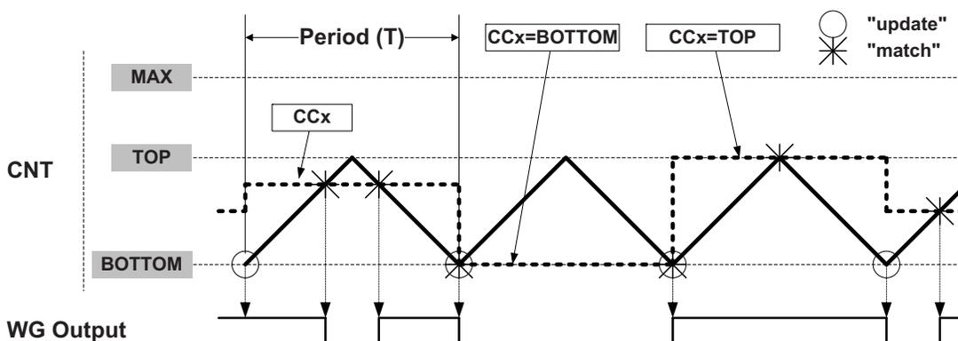
Using dual-slope PWM results in a lower maximum operation frequency compared to the single-slope PWM operation. The period register (PER) defines the PWM resolution. The minimum resolution is 2 bits (PER=0x0003), and the maximum resolution is 16 bits (PER=MAX).
