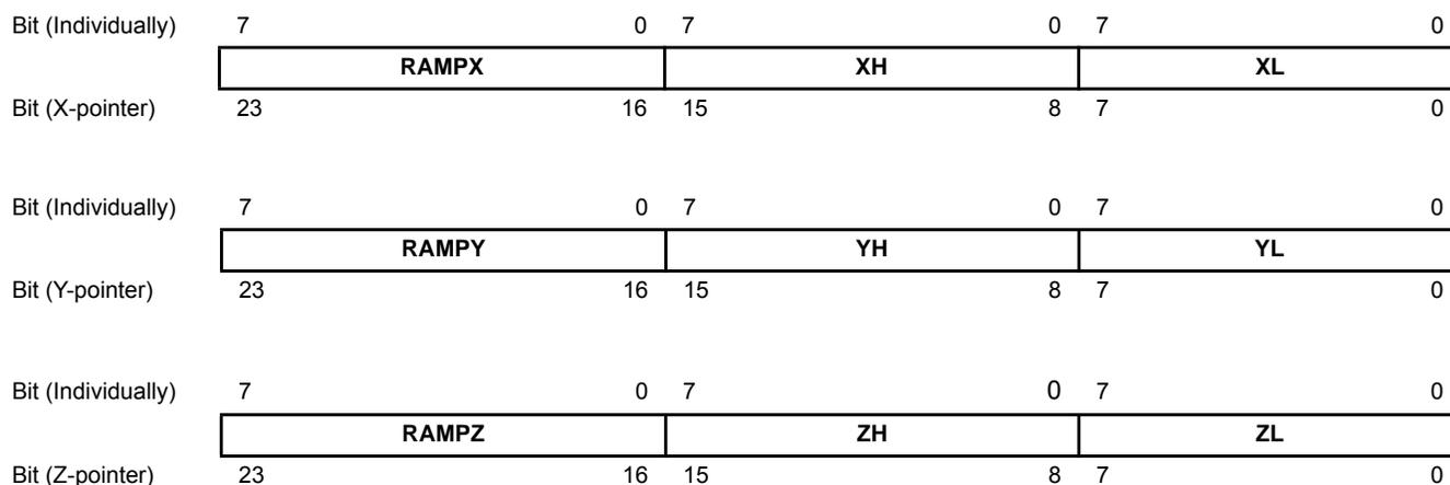
When reading (ELPM) and writing (SPM) program memory locations above the first 128KB of the program memory, RAMPZ is concatenated with the Z-register to form the 24-bit address. LPM is not affected by the RAMPZ setting.
