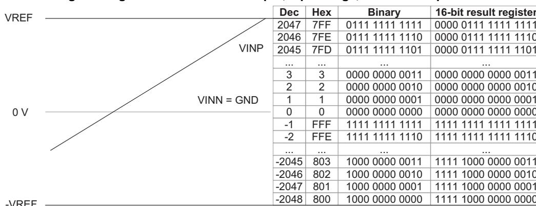
**Figure 26-11. Unsigned single-ended and internal input, input range, and result representation.**
