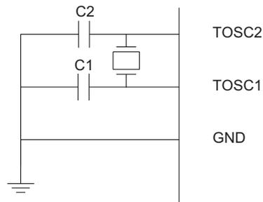
Two capacitors, C1 and C2, may be added to match the required load capacitance for the connected crystal. For details on recommended TOSC characteristics and capacitor load, refer to device datasheets.
