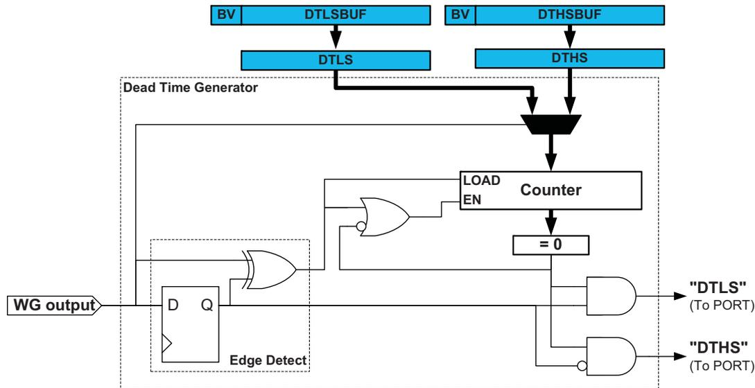
As shown in Figure 15-4 on page 188, the 8-bit dead-time counter is decremented by one for each peripheral clock cycle, until it reaches zero. A nonzero counter value will force both the low side and high side outputs into their OFF state. When a change is detected on the WG output, the dead-time counter is reloaded according to the edge of the input. A positive edge initiates a counter reload of the DTLS register, and a negative edge a reload of DTHS register.
