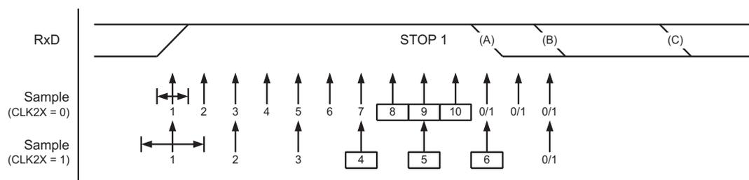
A new high-to-low transition indicating the start bit of a new frame can come right after the last of the bits used for majority voting. For normal speed mode, the first low level sample can be at the point marked (A) in Stop Bit Sampling and Next Start Bit Sampling. For double speed mode, the first low level must be delayed to point (B). Point (C) marks a stop bit of full length at nominal baud rate. The early start bit detection influences the operational range of the receiver.
