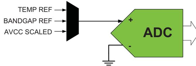
To measure the internal signals in unsigned mode, the negative input is connected to a fixed value given by the formula below, which is half of the voltage reference (VREF) minus a fixed offset, as it is for single-ended unsigned input. Refer to [Figure 26-11 on page 326](#) for details.
