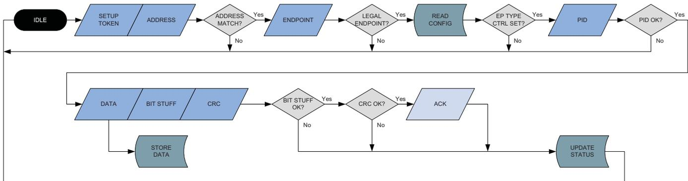
The USB module then fetches the endpoint data pointer register (DATAPTR) and waits for a DATA0 packet. If a PID error or any other PID than DATA0 is detected, the USB module returns to idle and waits for the next token packet.
