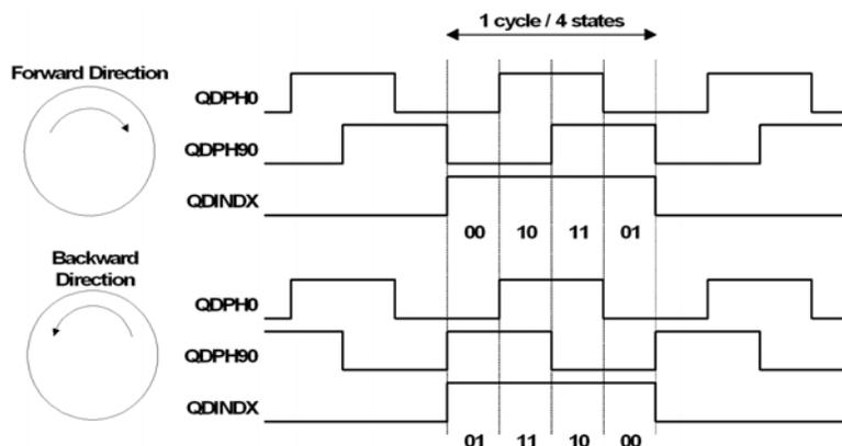
[Figure 6-4](#) shows typical quadrature signals from a rotary encoder. The signals QDPH0 and QDPH90 are the two quadrature signals. When QDPH90 leads QDPH0, the rotation is defined as positive or forward. When QDPH0 leads QDPH90, the rotation is defined as negative or reverse. The concatenation of the two phase signals is called the quadrature state or the phase state.
