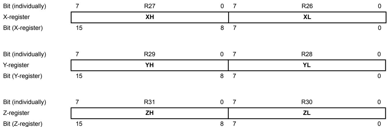
The lowest register address holds the least-significant byte (LSB), and the highest register address holds the most-significant byte (MSB). In the different addressing modes, these address registers function as fixed displacement, automatic increment, and automatic decrement (see the instruction set reference for details).
