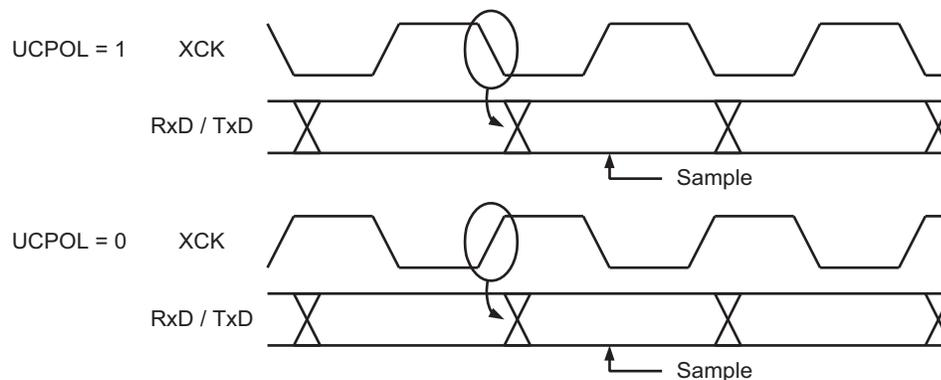
Using the inverted I/O (INVEN) setting for the corresponding XCK port pin, the XCK clock edges used for data sampling and data change can be selected. If inverted I/O is disabled (INVEN=0), data will be changed at the rising XCK clock edge and sampled at the falling XCK clock edge. If inverted I/O is enabled (INVEN=1), data will be changed at the falling XCK clock edge and sampled at the rising XCK clock edge. For more details, see “I/O Ports” on page 123.
