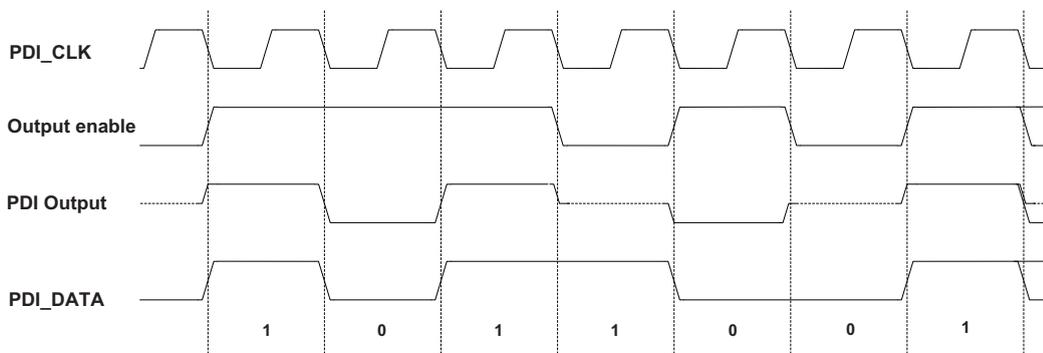
If the programmer and the PDI both drive the PDI\_DATA line at the same time, drive contention will occur, as illustrated in Figure 29-9 on page 365. Every time a bit value is kept for two or more clock cycles, the PDI is able to verify that the correct bit value is driven on the PDI\_DATA line. If the programmer is driving the PDI\_DATA line to the opposite bit value to what the PDI expects, a collision is detected.
