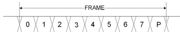
**(0-7)** Data/command bits, least-significant bit sent first (0 to 7)
