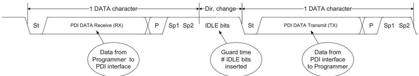
The external programmer will lose control of the PDI\_DATA line at the point where the PDI changes from RX to TX mode. The guard time relaxes this critical phase of the communication. When the programmer changes from RX mode to TX mode, a single IDLE bit, at minimum, should be inserted before the start bit is transmitted.
