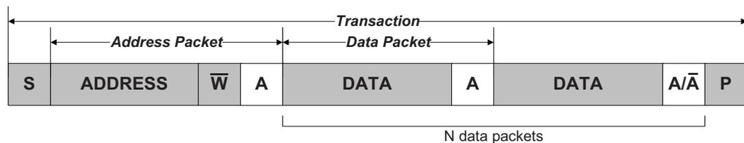
Assuming the slave acknowledges the address, the master can start transmitting data (DATA) and the slave will ACK or NACK ( $A/\bar{A}$ ) each byte. If no data packets are to be transmitted, the master terminates the transaction by issuing a STOP condition (P) directly after the address packet. There are no limitations to the number of data packets that can be
