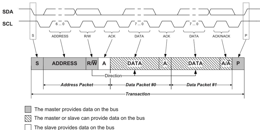
The master provides the clock signal for the transaction, but a device connected to the bus is allowed to stretch the low-level period of the clock to decrease the clock speed.
