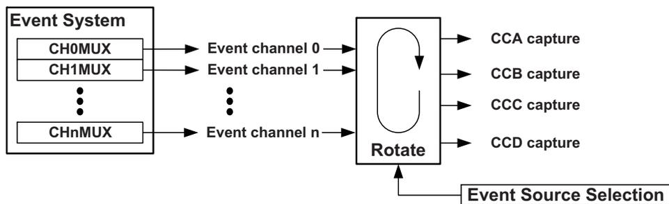
The event action setting in the timer/counter will determine the type of capture that is done.
