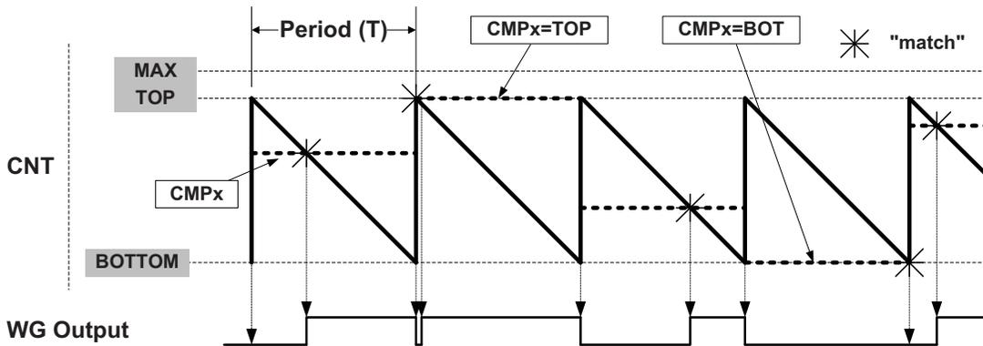
The PER register defines the PWM resolution. The minimum resolution is two bits (PER=0x0003), and the maximum resolution is eight bits (PER=MAX).
