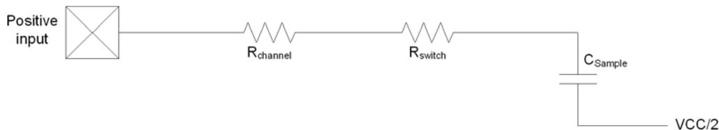
Figure 26-19. ADC input for differential measurements and differential measurements with gain.
