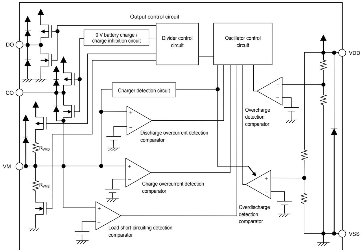
**Remark** All diodes shown in figure are parasitic diodes.
