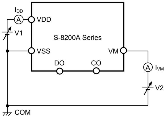
Figure 7 Test Circuit 3
