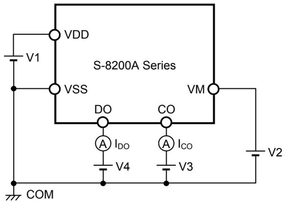
Figure 8 Test Circuit 4
