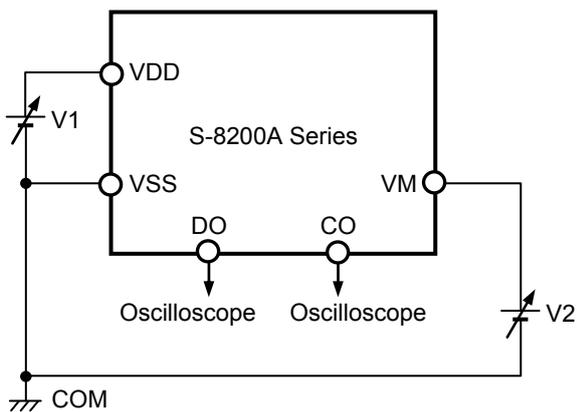
Figure 9 Test Circuit 5
