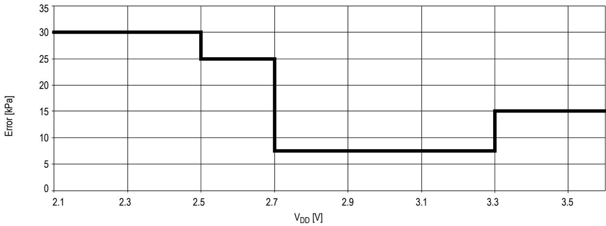
**Figure 10. Pressure Error vs V<sub>DD</sub> at T = 25°C, 250 kPa ≤ P ≤ 450 kPa**
