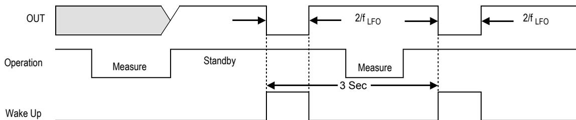
**Figure 3. Pulse on OUT Pin During Standby Mode**
