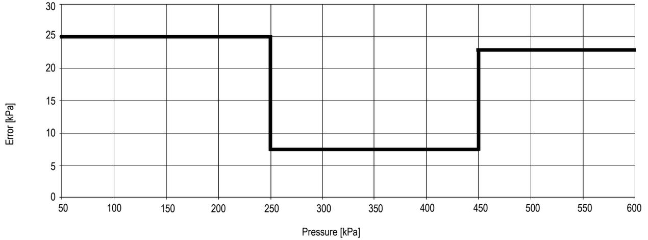
**Figure 9. Pressure Error vs Pressure at T = 25°C, 2.7 V ≤ V<sub>DD</sub> ≤ 3.3 V**
