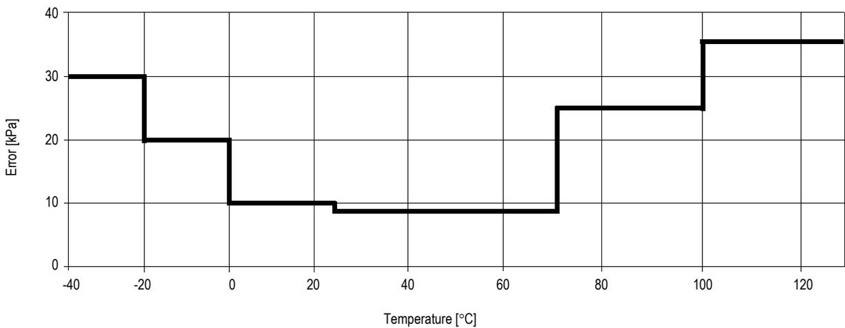
**Figure 11. Pressure Error vs Temperature at V<sub>DD</sub> = 3.0 V, 250 kPa ≤ P ≤ 450 kPa**
