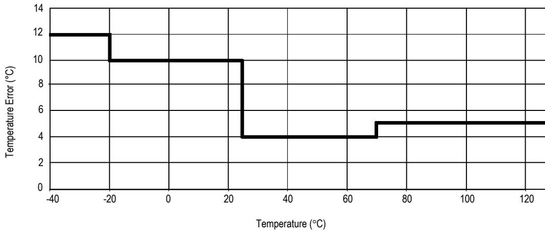
**Figure 7. Temperature Error vs Temperature at V<sub>DD</sub> = 3.0 V**
