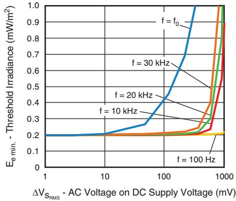
Fig. 7 - Sensitivity vs. Supply Voltage Disturbances
