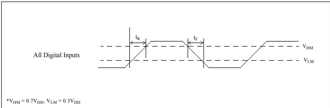
**Figure 16 - Digital Signal Input Rise/Fall Times**
