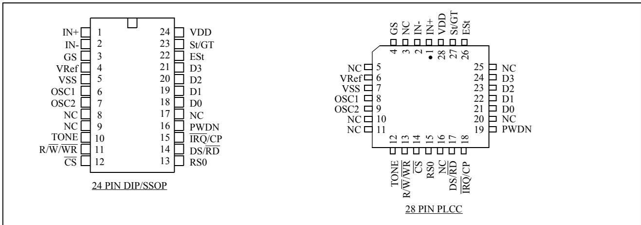
Figure 2 - Pin Connections
