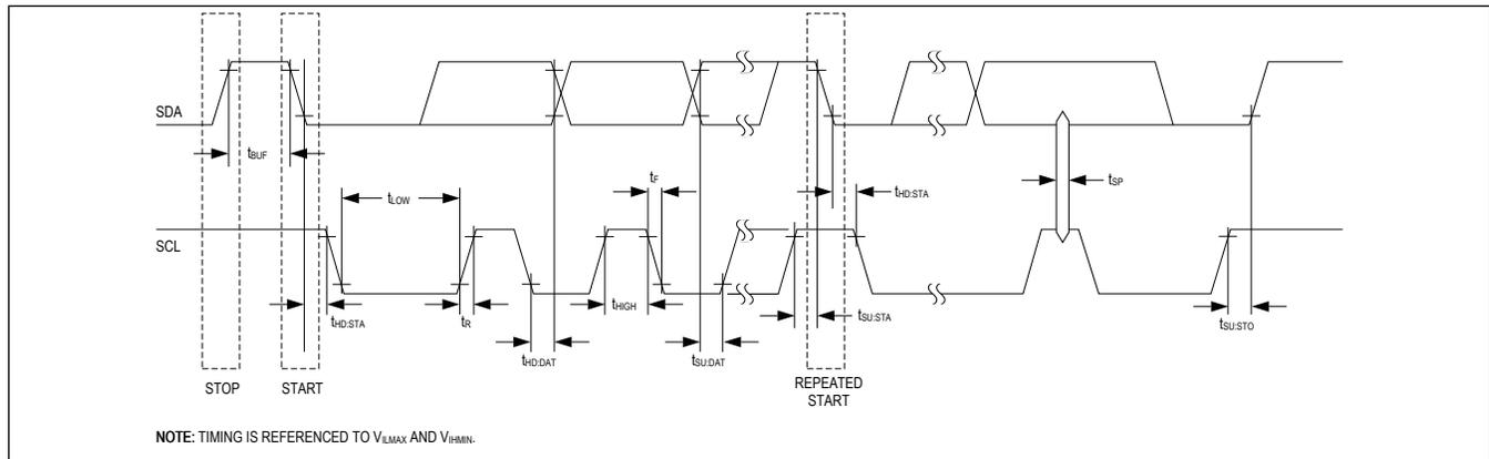
Figure 1. Data Transfer on I<sup>2</sup>C Serial Bus
