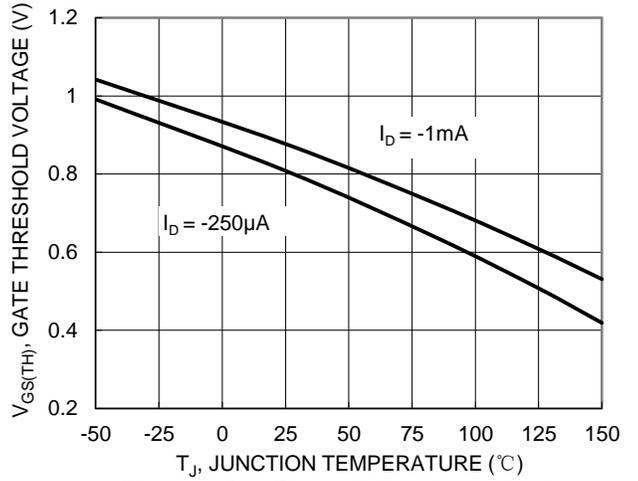
Figure 20. Gate Threshold Variation vs. Junction Temperature
