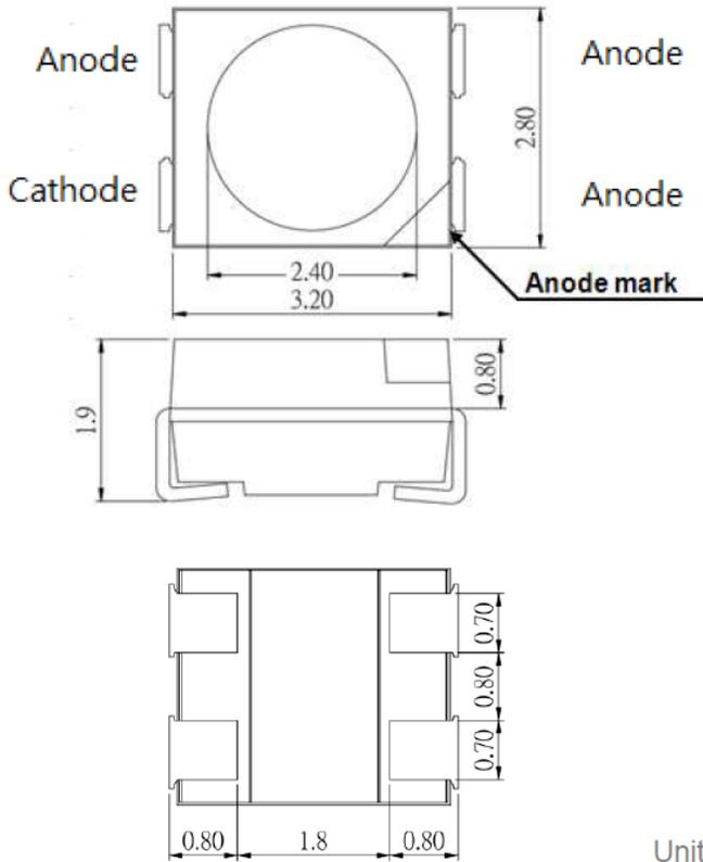
Unit: mm, Tolerance:  $\pm 0.1\text{mm}$
