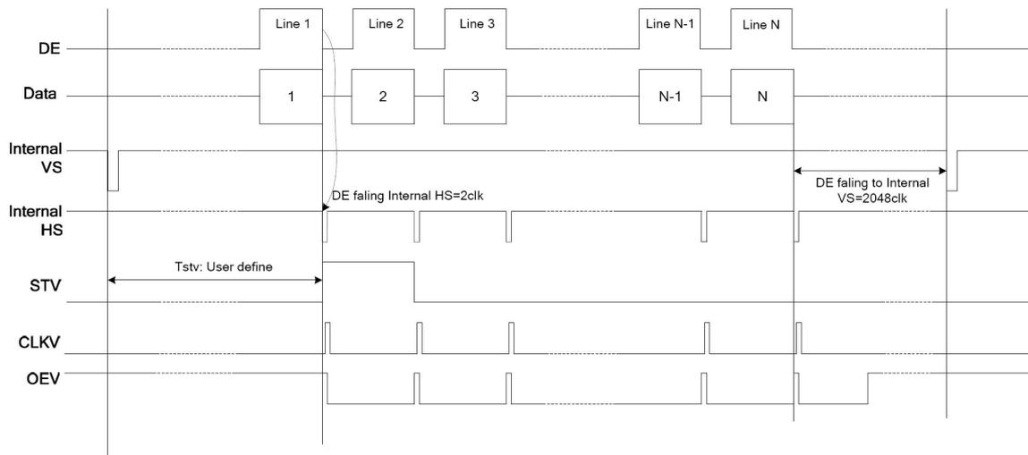
**Input Data Timing (24 bit RGB mode for 960×240 @ SEL[3:0]=1100b)**
