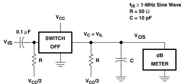
**Figure 7. Switch OFF Signal Feedthrough Test Circuit**
