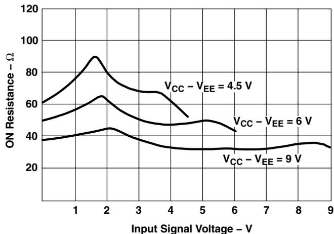
**Figure 9. Typical ON Resistance vs Input Signal Voltage**
