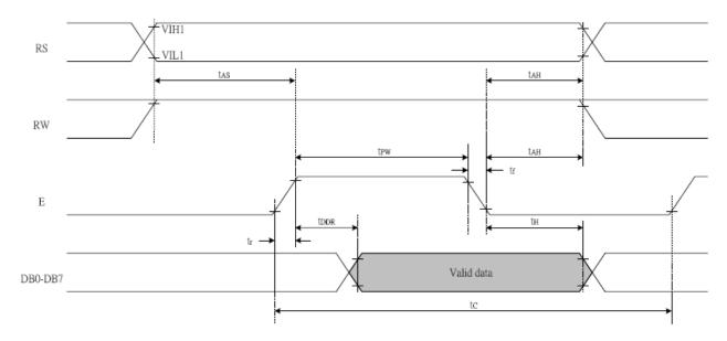
Write cycle (Ta=25°C, VDD=3.0V)
