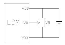
$V_{\text{DD-}}V_0$ : LCD Driving voltage
