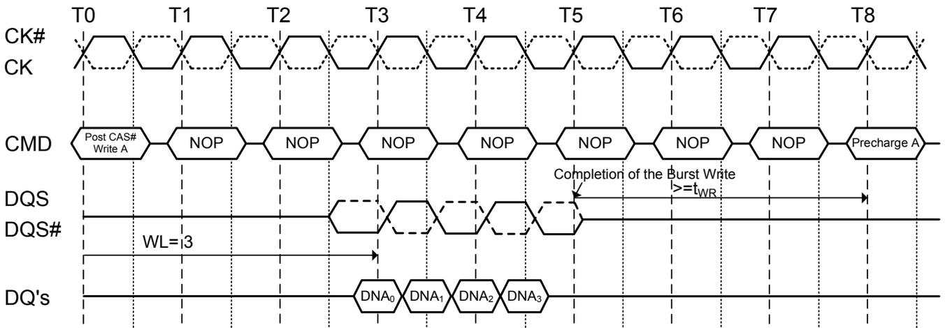
**Figure 31.2. Burst write followed by precharge:  $WL = (RL-1) = 4$**
