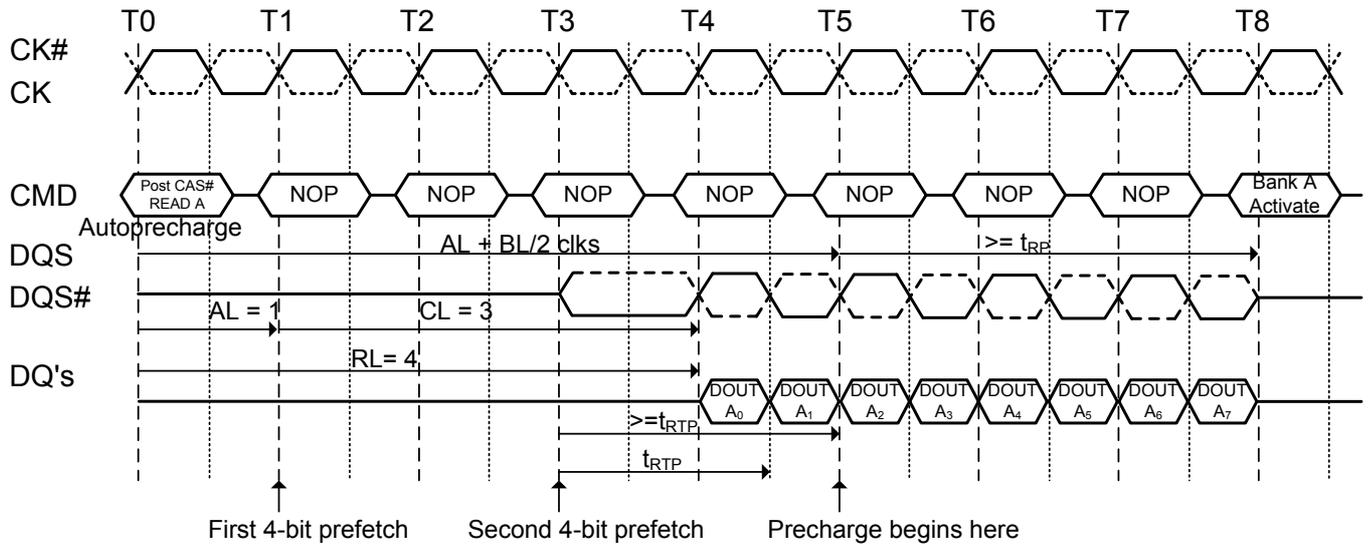
**Figure 32.2. Burst read operation with auto precharge:
