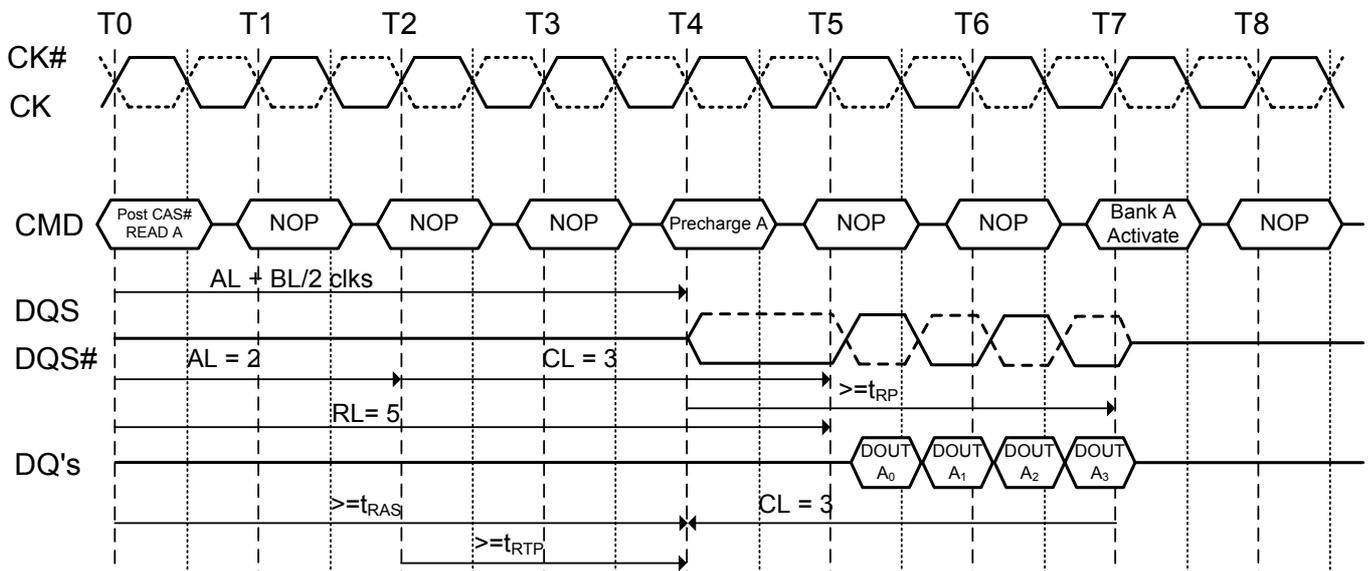
**Figure 30.4. Burst read operation followed by precharge:**
