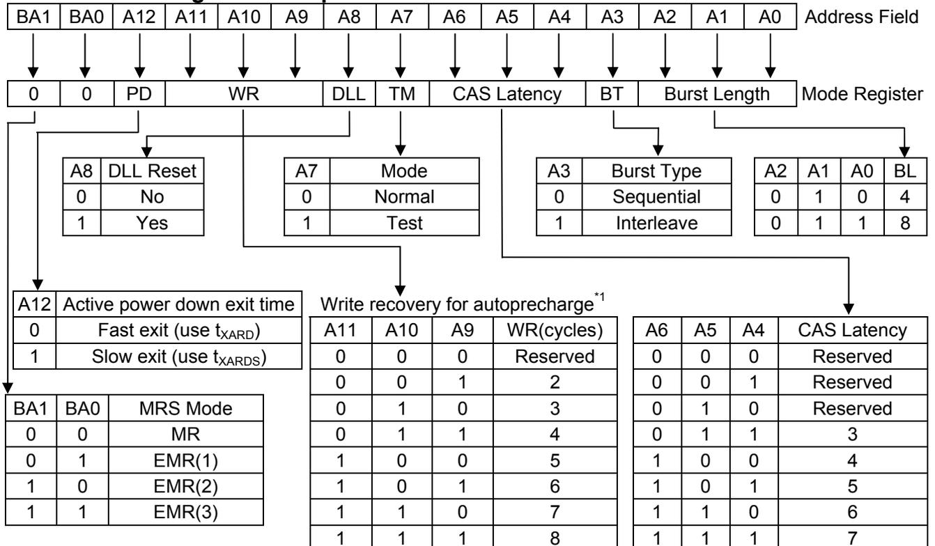
**Note 1:** For DDR2-800, WR (write recovery for autoprecharge) min is determined by  $t_{CK} (avg)$  max and WR max is determined by  $t_{CK}(avg)$  min.  $WR [cycles] = RU \{t_{WR}[ns]/t_{CK}(avg)[ns]\}$ , where RU stands for round up. The mode register must be programmed to this value. This is also used with  $t_{RP}$  to determine  $t_{DAL}$ .
