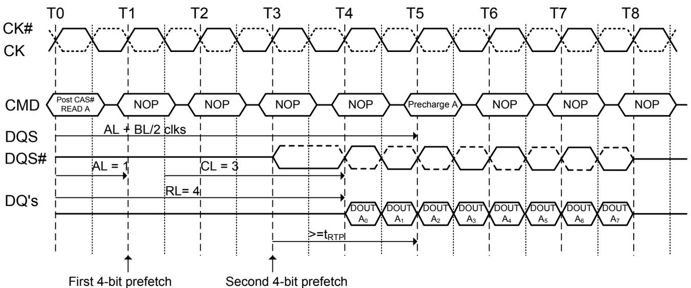
**Figure 30.3. Burst read operation followed by precharge:**
