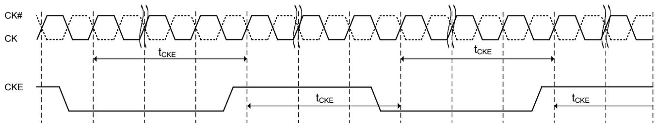
NOTE: DRAM guarantees all AC and DC timing & voltage specifications and proper DLL operation with intensive CKE operation
