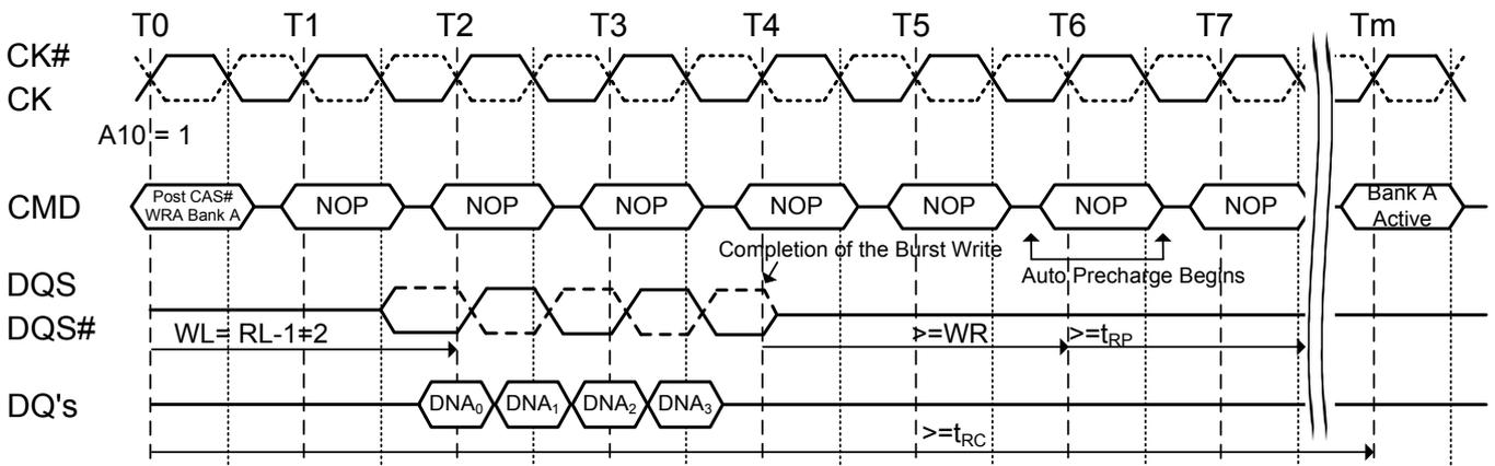
**Figure 33.2. Burst write with auto-precharge (WR+t<sub>RP</sub>): WL=4, WR=2, BL=4, t<sub>RP</sub>=3**
