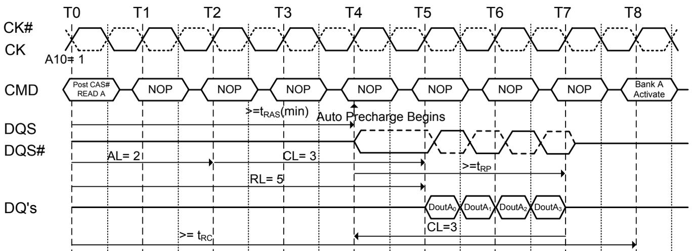
**Figure 32.4. Burst read operation with auto precharge followed by an activation to the same bank ( $t_{RP}$  Limit): (RL=5 (AL=2, CL=3, internal  $t_{RCD}$ =3, BL=4,  $t_{RTP}$  2 clocks)**
