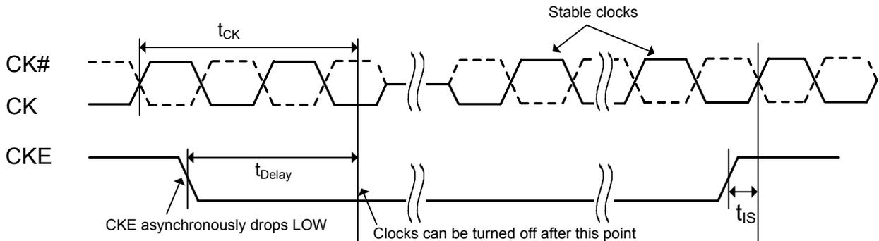
**Figure 47. Clock frequency change in precharge power down mode**
