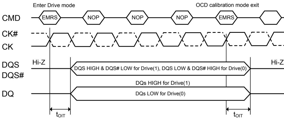
NOTE : Drive mode, both Drive(1) and Drive(0), is used for controllers to measure DDR2 SDRAM Driver impedance. In this mode, all outputs are driven out  $t_{OIT}$  after "enter drive mode" command and all output drivers are turned-off  $t_{OIT}$  after "OCD calibration mode exit" command.
