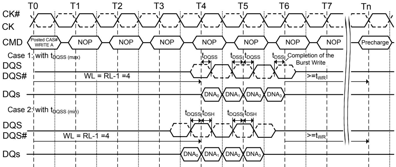
**Figure 25.2. Burst write operation: RL=3 (AL=0, CL=3), WL=2, BL=4**
