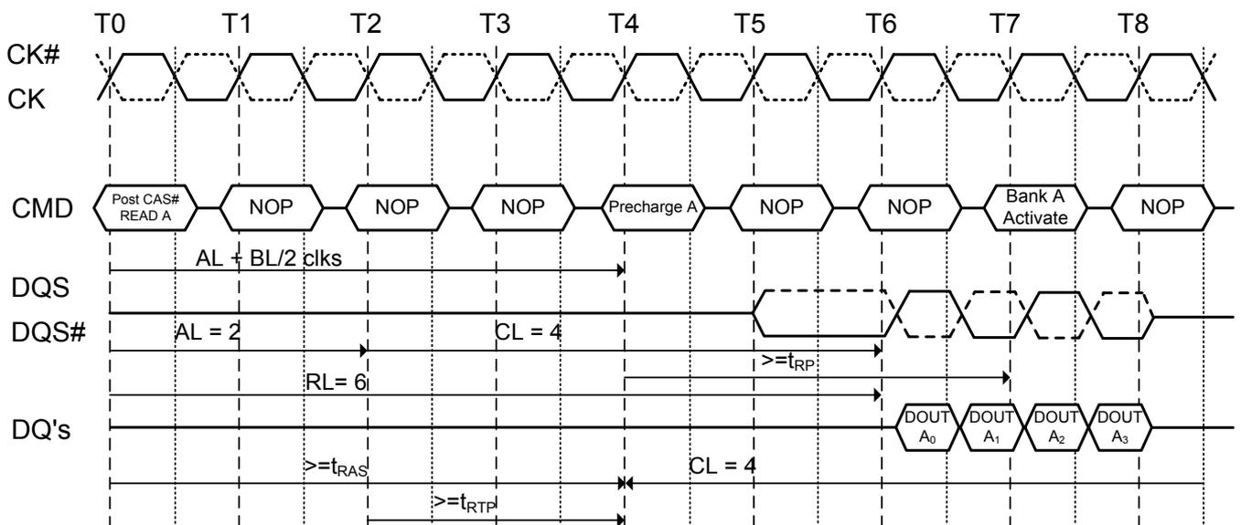
**Figure 30.5. Burst read operation followed by precharge:**
