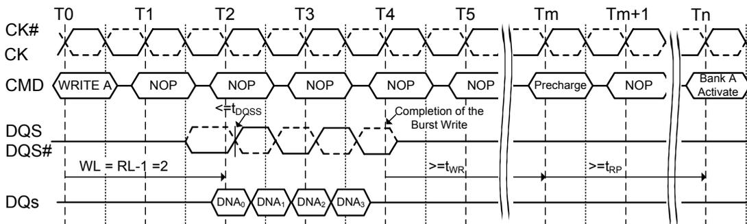
**Figure 26. Burst write followed by burst read:
