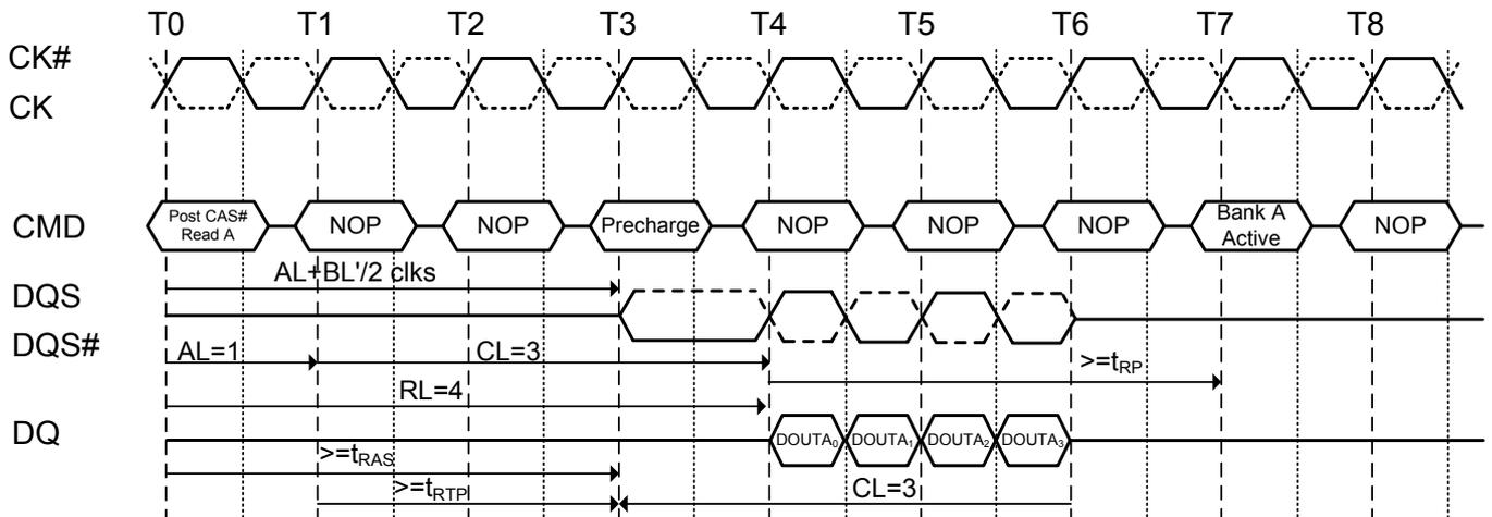
**Figure 30.2. Burst read operation followed by precharge:**
