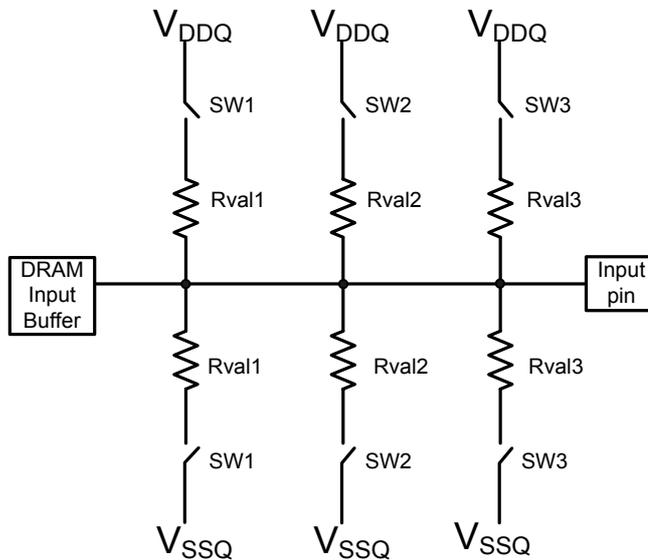
Switch (sw1, sw2, sw3) is enabled by ODT pin.
