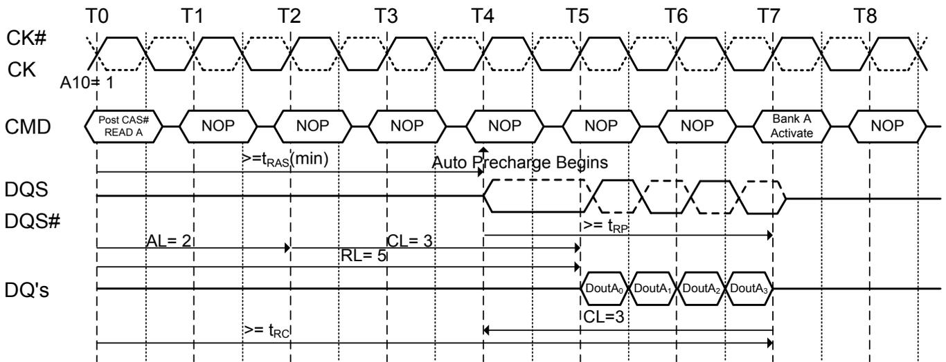
**Figure 33.1. Burst write with auto-precharge ( $t_{RC}$  Limit): WL=2, WR=2, BL=4,  $t_{RP}$ =3**
