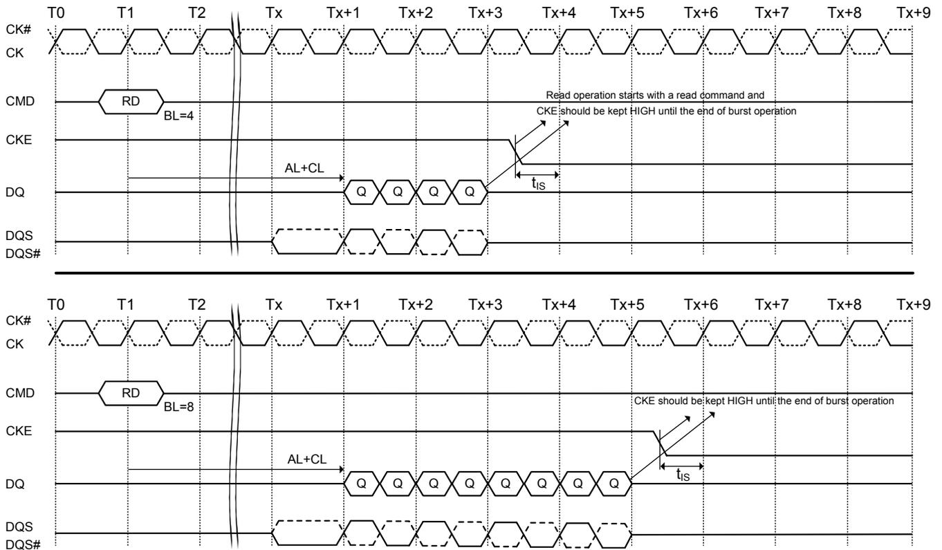
**Figure 39. Read with autoprecharge to power-down entry**
