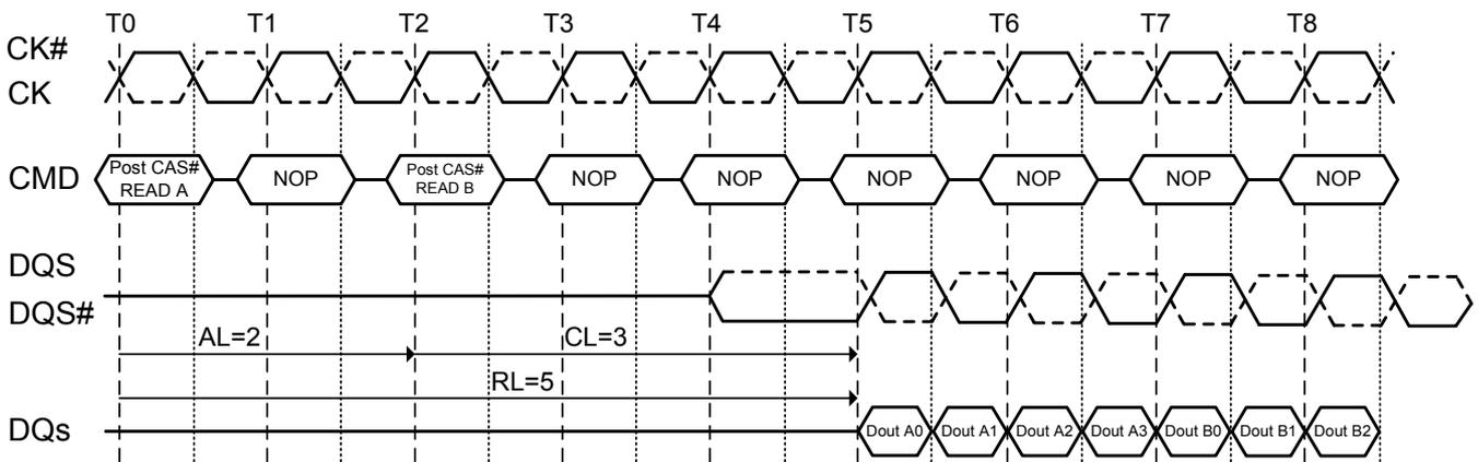
**NOTE :** The seamless burst read operation is supported by enabling a read command at every other clock for BL = 4 operation, and every 4 clock for BL =8 operation. This operation is allowed regardless of same or different banks as long as the banks are activated.
