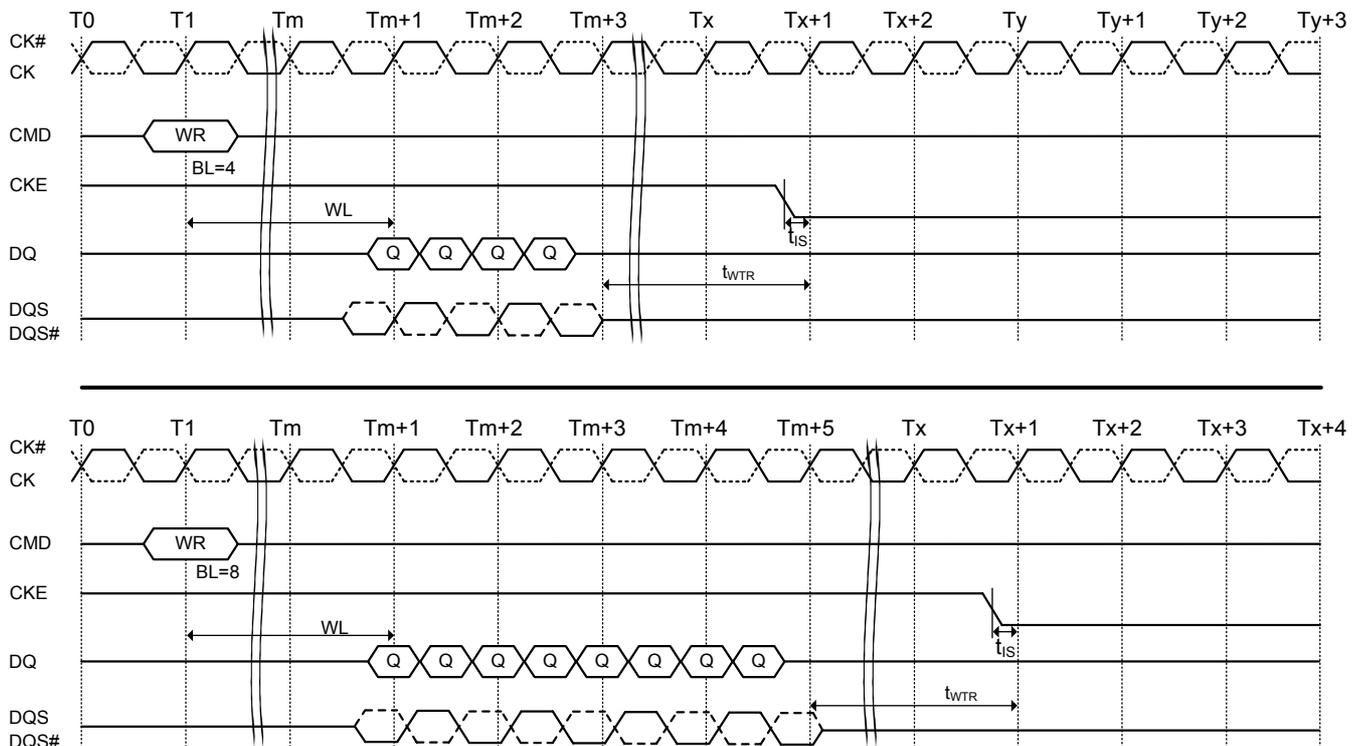
**Figure 44. Precharge/precharge-all command to power-down entry**
