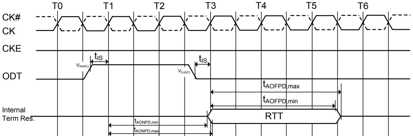
**Figure 15. ODT timing mode switch at entering power-down mode**
