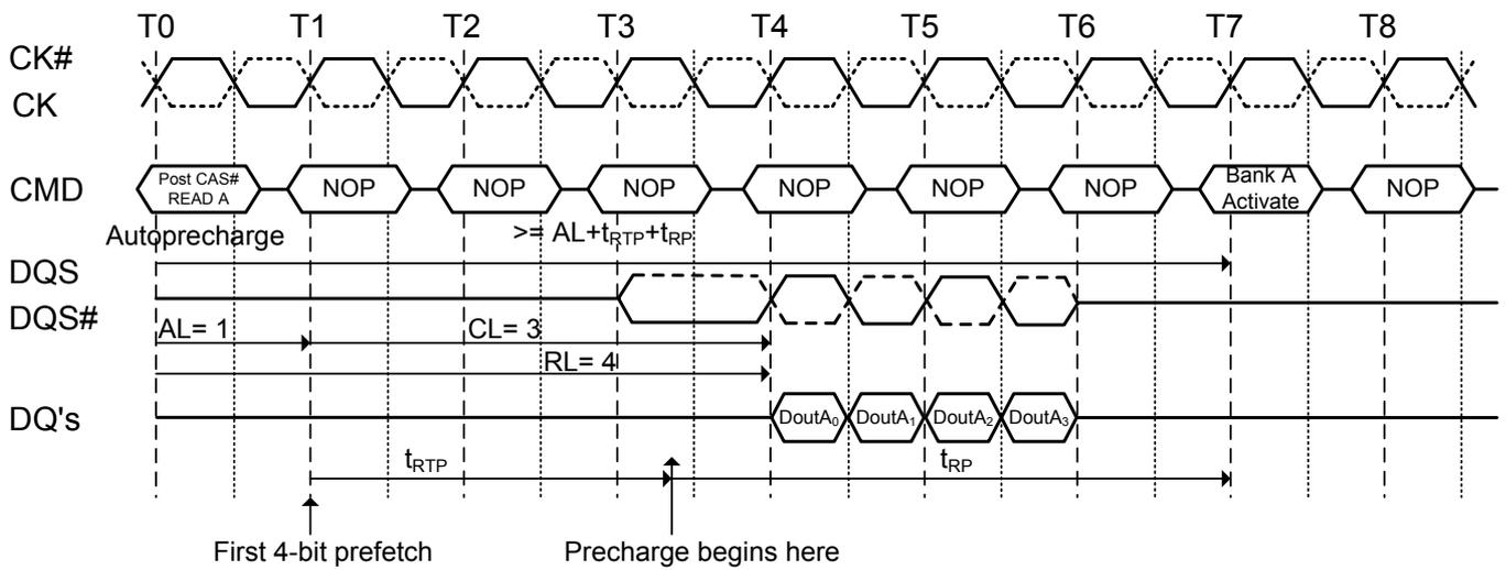
**Figure 32.3. Burst read operation with auto precharge followed by activation to the same bank ( $t_{RC}$  Limit): RL=5(AL=2, CL=3, internal  $t_{RCD}=3$ , BL=4,  $t_{RTP} = 2$  clocks)**
