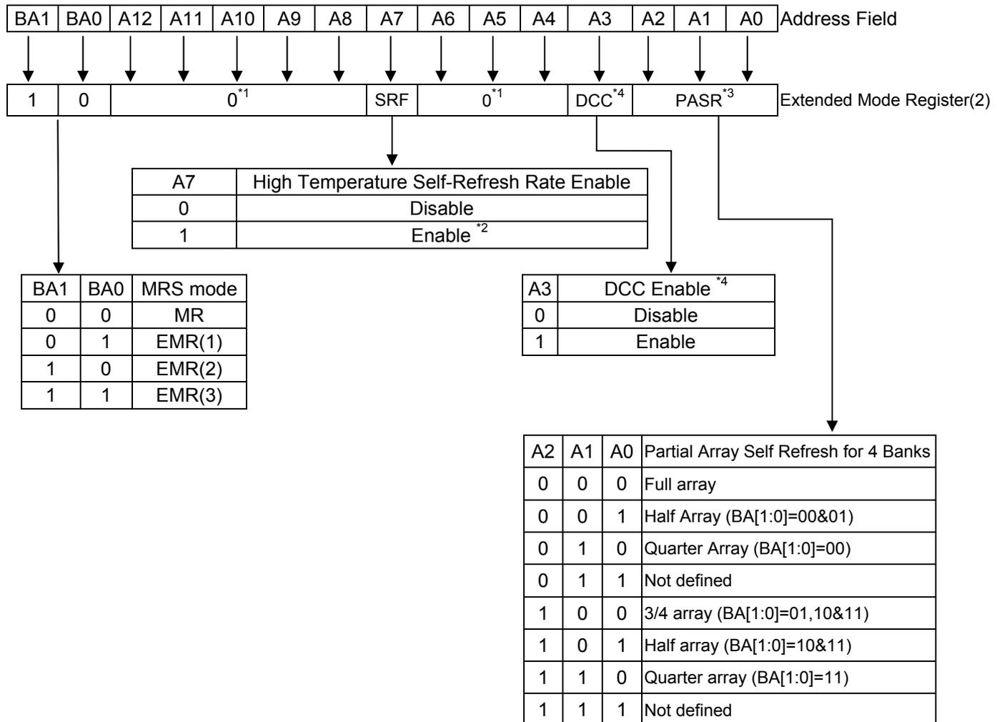
**NOTE 1:** The rest bits in EMRS(2) are reserved for future use and all bits in EMRS(2) except A0-A2, A7, BA0 and BA1 must be programmed to 0 when setting the extended mode register(2) during initialization.
