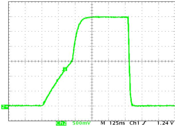
Figure 10. SIM\_IO Typical Rise and Fall Times with Stray Capacitance > 30 pF (33 pF Capacitor Connected on the Board)
