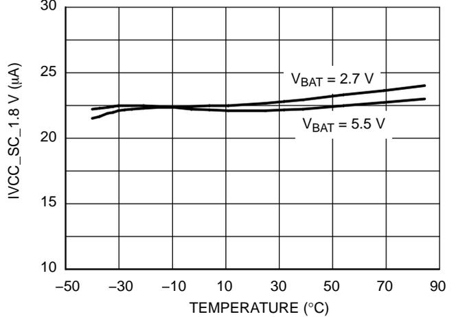
Figure 7.  $I_{BAT}$  vs Temperature at 1.8 V
