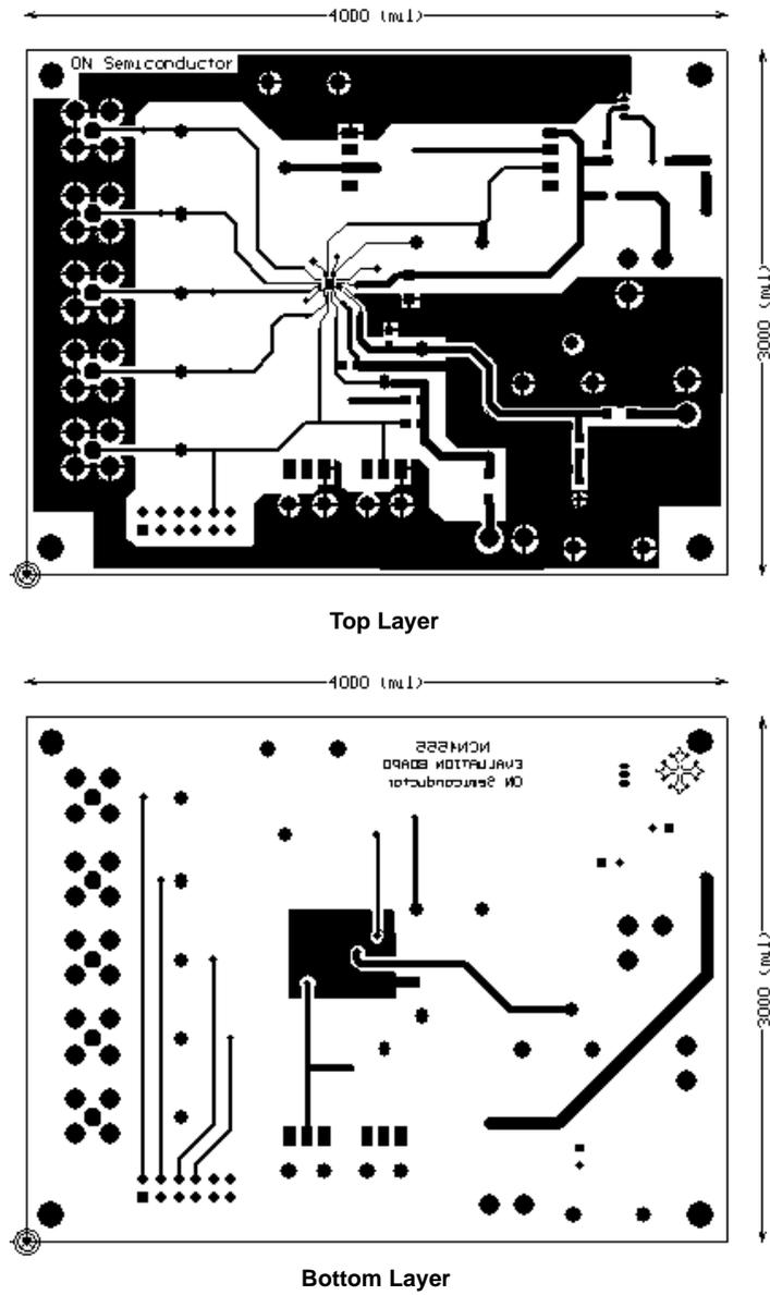
Figure 13. NCN4555 Printed Circuit Board Layout (Engineering board)
