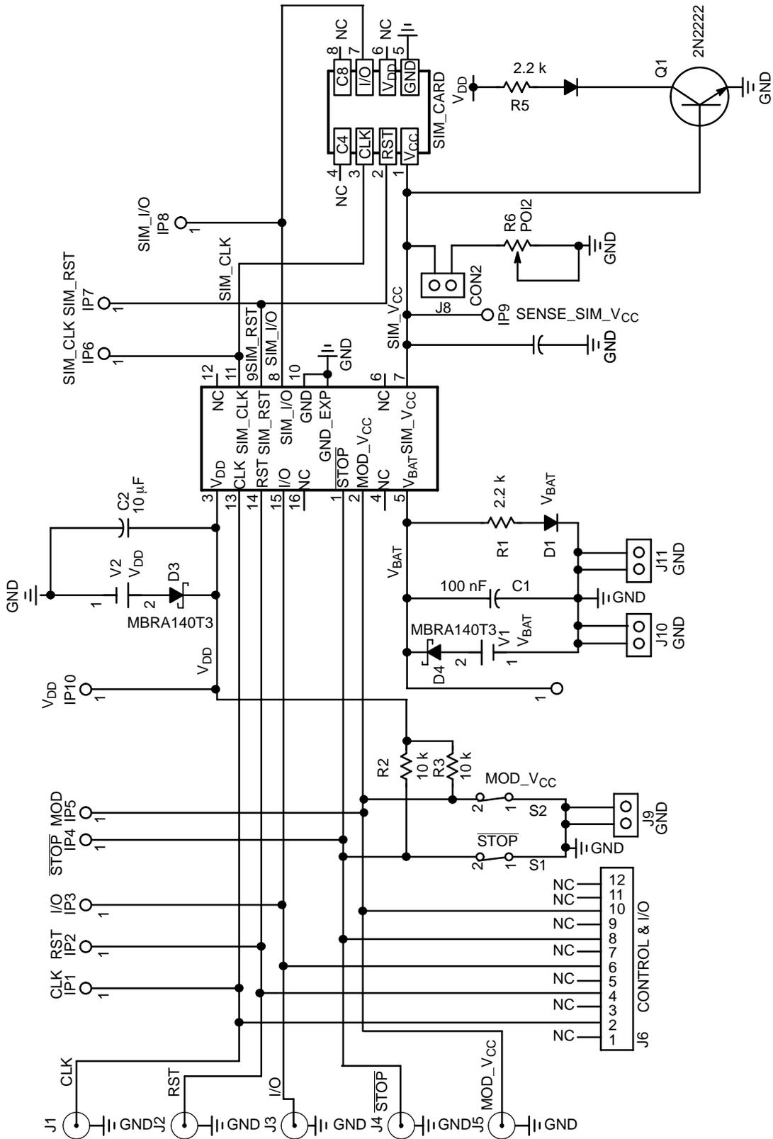
Figure 12. NCN4555 engineering test board schematic diagram
