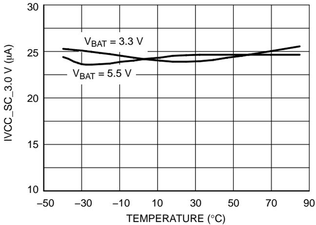
Figure 6.  $I_{BAT}$  vs temperature at 3.0 V
