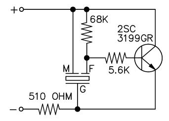
Notes: 1. The current consumption and the sound pressure level are measured by using the recommended driving circuit shown above.
