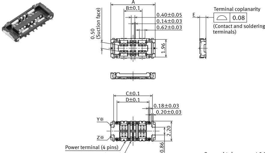
※ Because the soldering terminal Y and Z are the unified structure, they are connected electrically.
