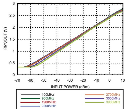
**RMSOUT Error vs. Pin with LTE 20MHz @ +25 °C** [1]
