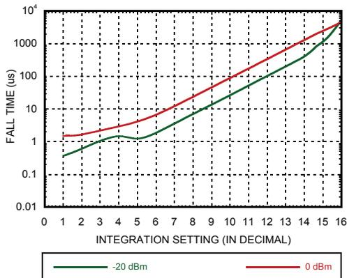
Figure 6. Fall Time<sup>[4]</sup> vs. SCI Setting over Input Power
