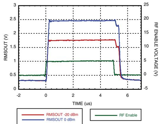
**RMSOUT Output Response with SCI = 1100 @ 1900 MHz [2]**
