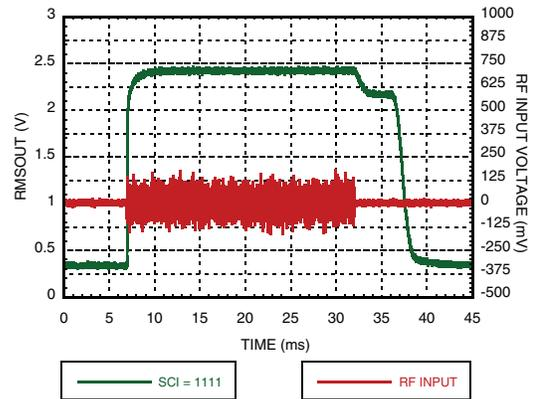
Figure 10. Residual Ripple for 1900 MHz
