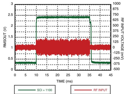
Figure 12. Residual Ripple for 1900 MHz
