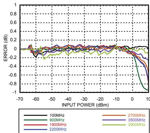
**RMSOUT Output Response with SCI = 0000 @ 1900 MHz [2]**
