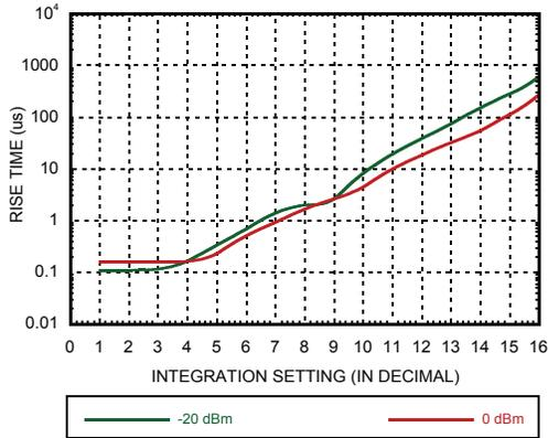
Figure 4. Rise Time<sup>[2]</sup> vs. SCI Setting over Input Power
