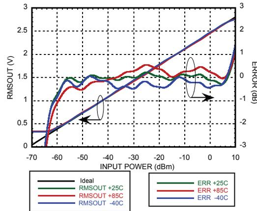
**RMSOUT & Error vs. Pin @ 1900 MHz** [1] [2]
