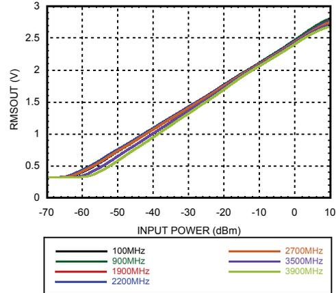
**RMSOUT Error vs. Pin with CW @ +25 °C [1]**
