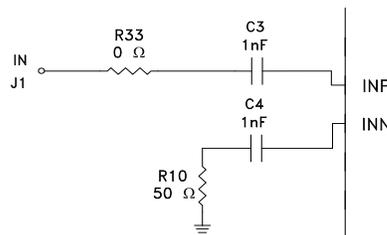
Note that the provided single-ended input interface covers the whole operating spectrum of the HMC1120LP4E and does not require matching/tuning for different frequencies. The performance of the HMC1120LP4E at different frequencies is shown below:
