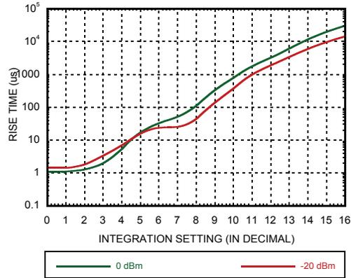
Figure 5. Rise Settling Time<sup>[3]</sup> vs. SCI Setting over Input Power
