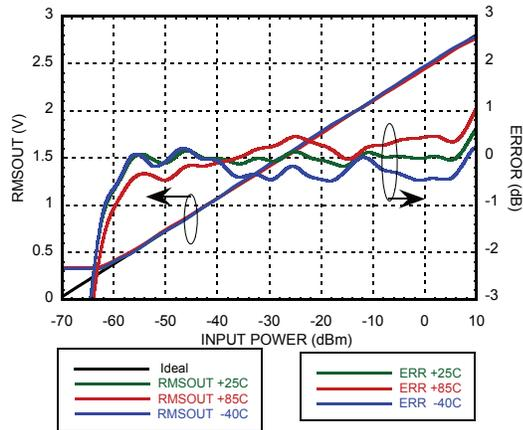
**RMSOUT & Error vs. Pin @ 900 MHz** [1] [2]
