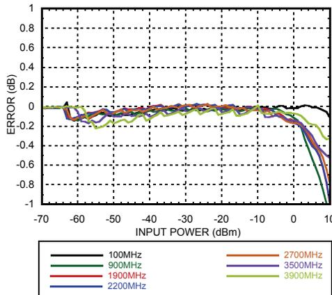
**RMSOUT vs. Pin w/ CW & LTE 20MHz @ 1900 MHz & +85 °C [1]**
