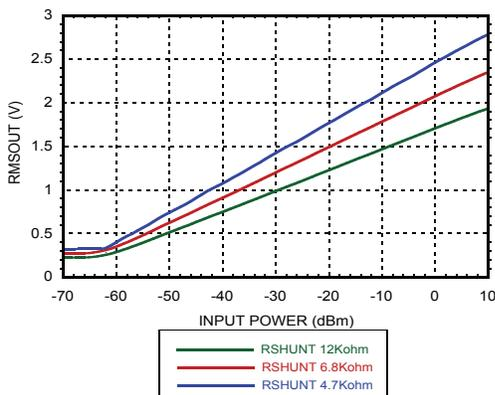
Figure 14. Slope Adjustment
