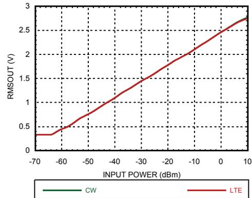
**Reading Error for LTE 20MHz wrt CW Response @ -40 °C [1]**
