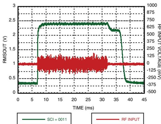
Figure 13. Residual Ripple for 1900 MHz
