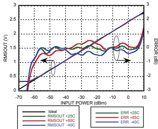
**RMSOUT & Error vs. Pin @ 3500 MHz** [1] [2]
