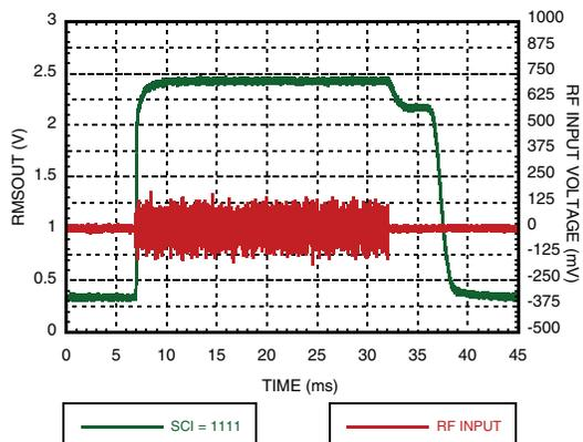
Figure 8. Residual Ripple for 1900 MHz WCDMA4C @ SCI=1111
