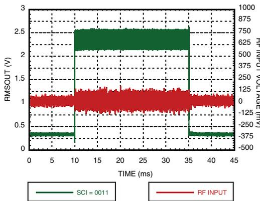
Figure 11. Residual Ripple for 1900 MHz
