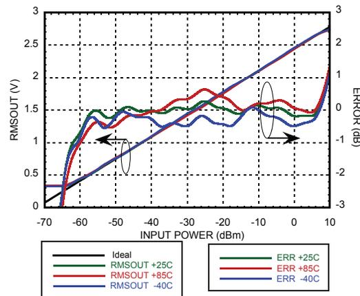
**RMSOUT & Error vs. Pin @ 2700 MHz** [1] [2]
