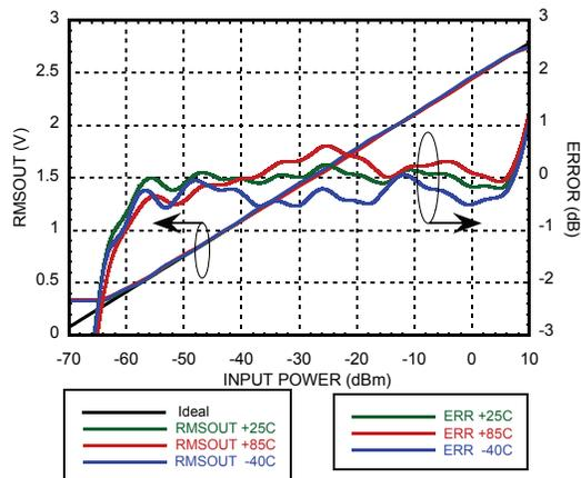
**RMSOUT & Error vs. Pin @ 2200 MHz** [1] [2]
