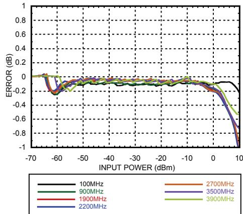
**RMSOUT vs. Pin w/ CW & LTE 20MHz @ 1900 MHz & -40 °C [1]**
