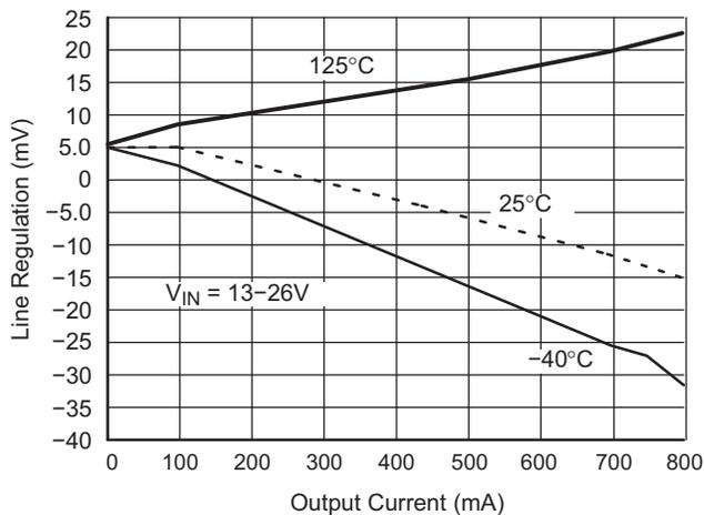
Figure 17. Line Regulation vs. Output Current for  $V_{OUT1}$
