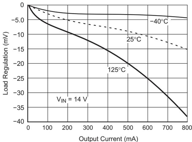
Figure 18. Load Regulation vs. Output Current for  $V_{OUT1}$
