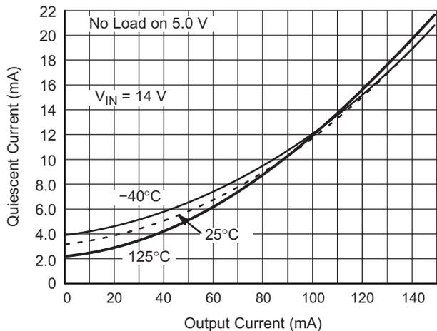
Figure 14. Quiescent Current vs. Output Current for  $V_{OUT1}$
