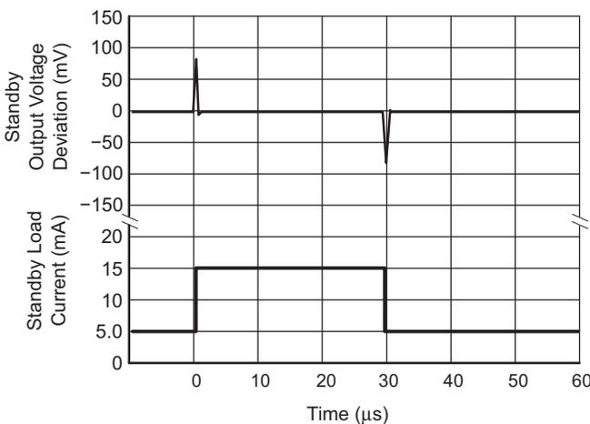
Figure 11. Load Transient Response ( $V_{OUT2}$ )
