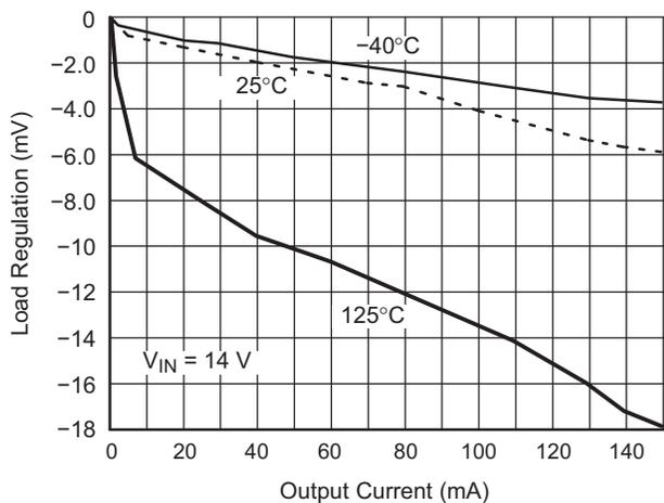
Figure 16. Load Regulation vs. Output Current for  $V_{OUT2}$
