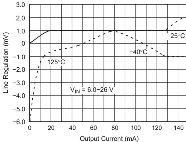
Figure 15. Line Regulation vs. Output Current for  $V_{OUT2}$
