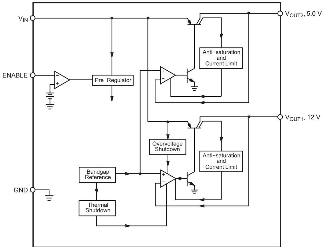
Figure 1. Block Diagram
