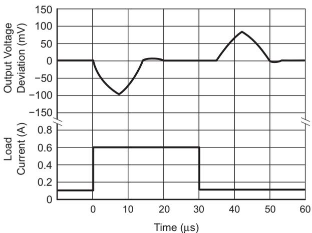
Figure 10. Load Transient Response ( $V_{OUT1}$ )
