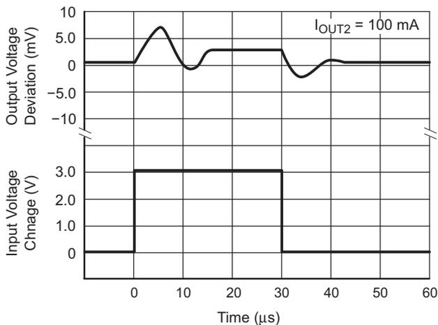
Figure 9. Line Transient Response ( $V_{OUT2}$ )
