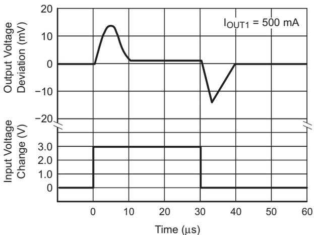
Figure 8. Line Transient Response ( $V_{OUT1}$ )
