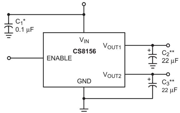
\*  $C_1$  is required if the regulator is far from power supply filter.
