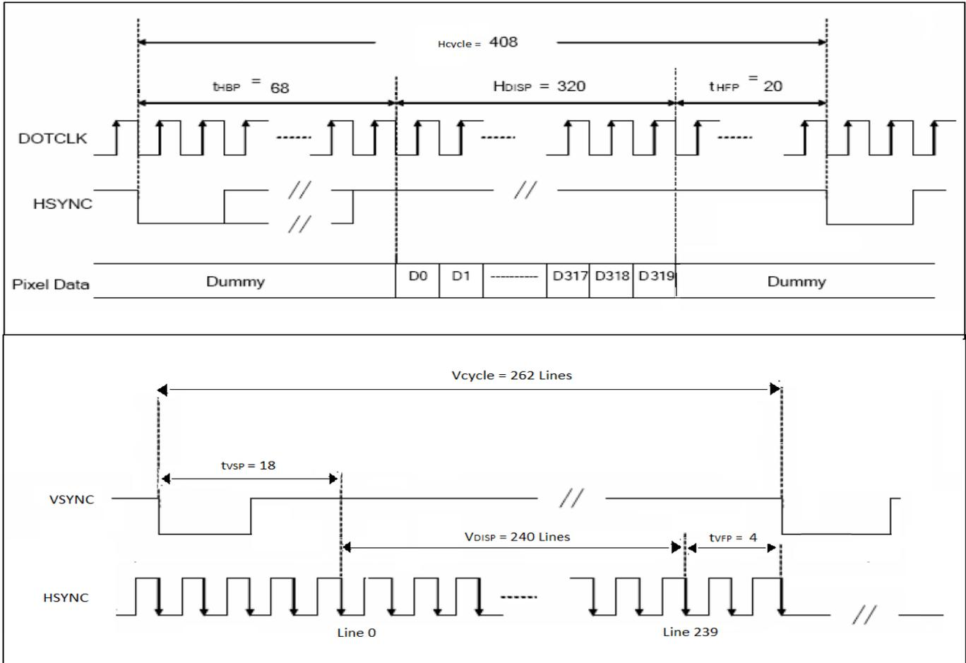
Figure 6.2: Vertical and Horizontal Data Transaction Timing Diagram
