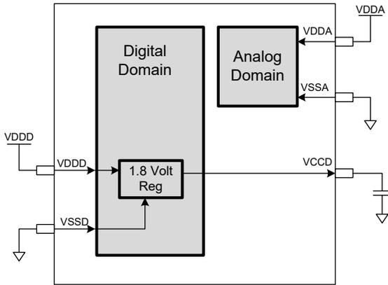
There are two distinct modes of operation. In Mode 1, the supply voltage range is 1.8 V to 5.5 V (unregulated externally; internal regulator operational). In Mode 2, the supply range is 1.8 V  $\pm$ 5% (externally regulated; 1.71 to 1.89, internal regulator bypassed).
