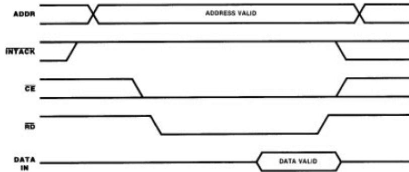
Figure 1. Z8500 Peripheral I/O Read Cycle Timing
