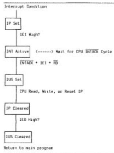
Figure 3. Z8500 Interrupt State Diagram
