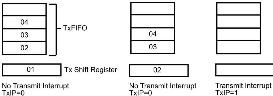
**Transmit Interrupt Status When WR7' D5=1 For ESCC**
