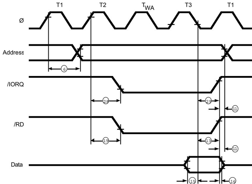
**Z180 I/O Read Cycle Timing (/IOC = 0)**
