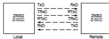
Figure 3. Block Diagram of Two Z8000 Development Modules
