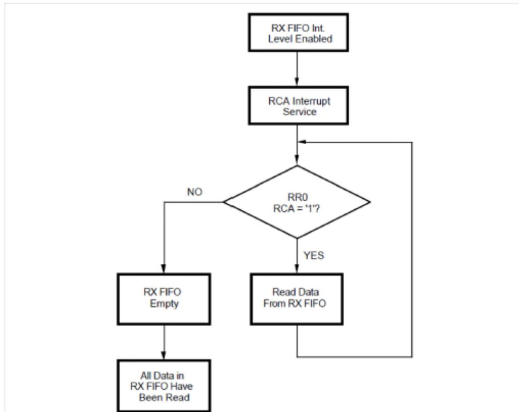
Figure 5. Flowchart of Receive Interrupt Service Routine to Reduce Receive Interrupt Frequencies
