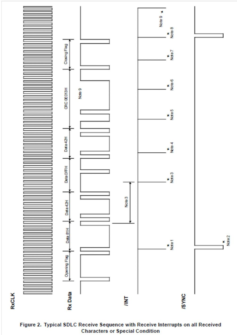
Figure 2. Typical SDLC Receive Sequence with Receive Interrupts on all Received Characters or Special Condition
