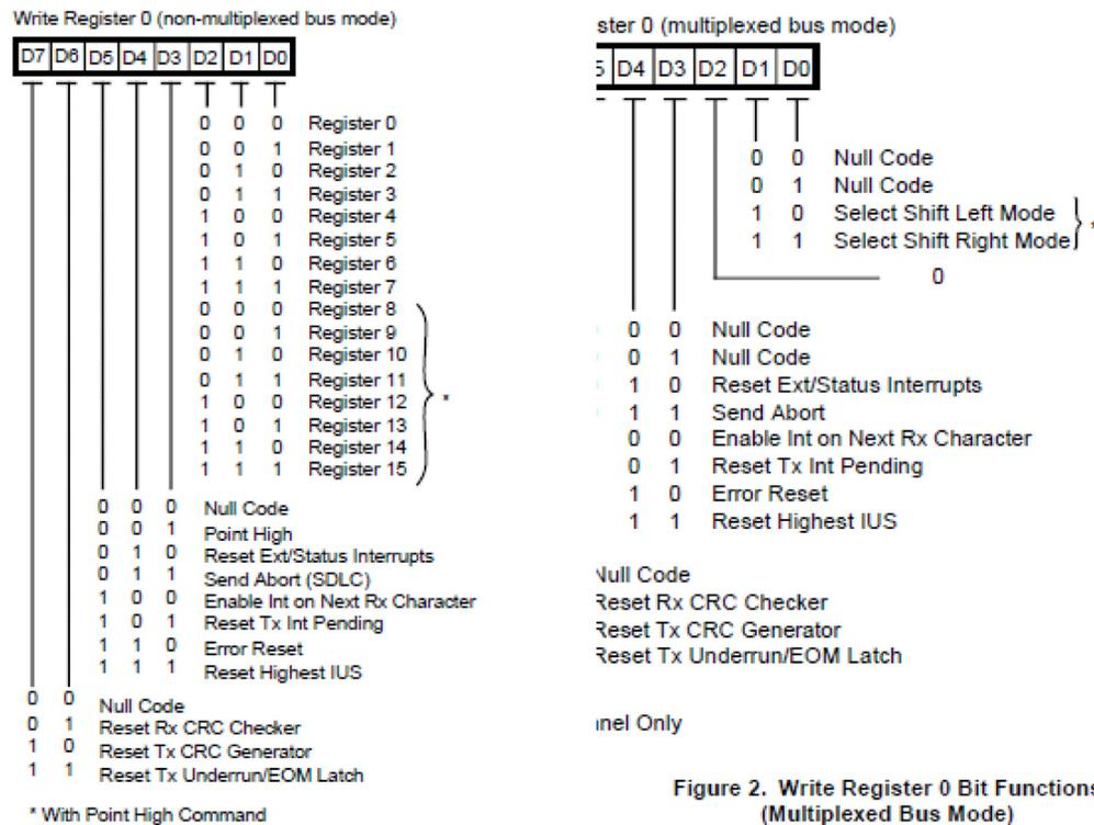
Figure 1. Write Register 0 Bit Functions (Non-Multiplexed Bus Mode)
