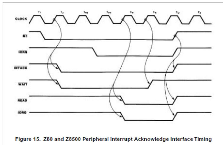
Figure 15. Z80 and Z8500 Peripheral Interrupt Acknowledge Interface Timing
