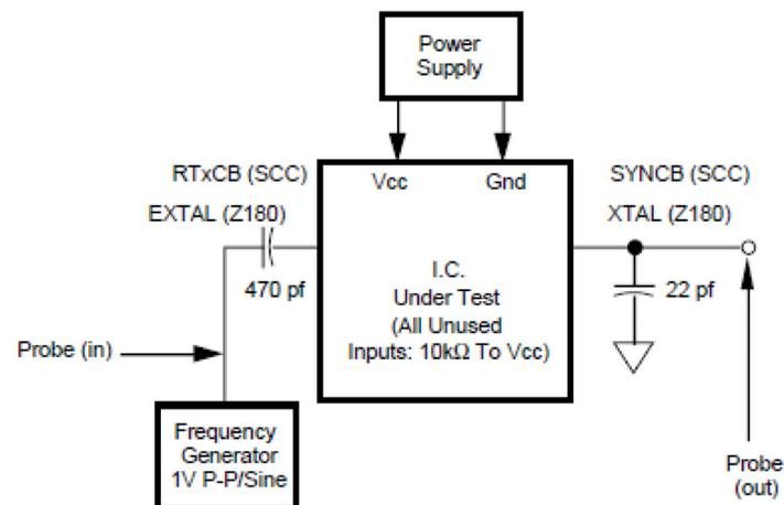
Figure 6. Gain Measurement
