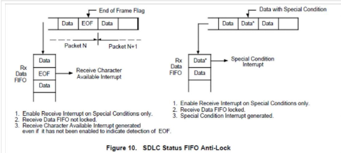
Figure 10. SDLC Status FIFO Anti-Lock
