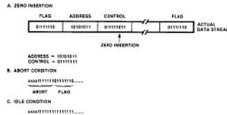
Figure 2. Bit Patterns for Various Line Conditions
