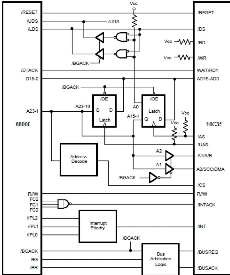
Figure 3. ISCC Interface to a 68000 Microprocessor
