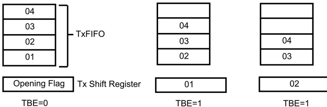
**Transmit Buffer Empty Bit Status For ESCC For Both WR7' and WR7' D5=0**
