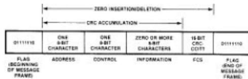
Figure 1. Fields of the SDLC Transmission Frame
