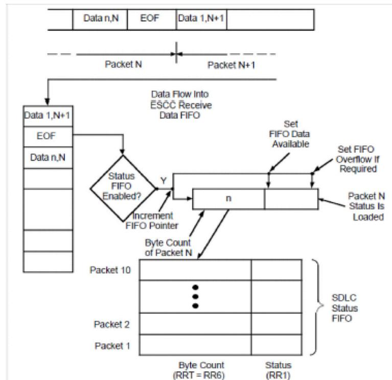
Figure 9. Status FIFO Operation at End Of Frame
