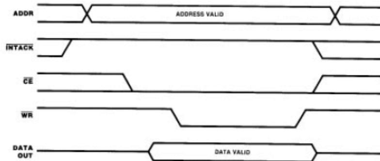
Figure 2. Z8500 Peripheral I/O Write Cycle Timing
