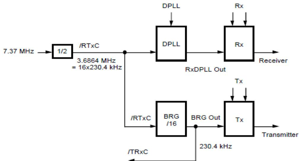
Figure 3. SCC Clocking Scheme
