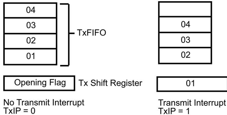
**Transmit Interrupt Status When WR7' D5=0 For ESCC**
