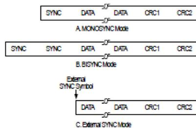
Figure 1. Synchronous Modes of Communication
