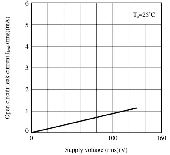
**Fig.8-b Open Circuit Leak Current vs. Supply Voltage (S202S11)**
