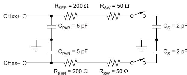
Figure 1. Equivalent Input Circuit
