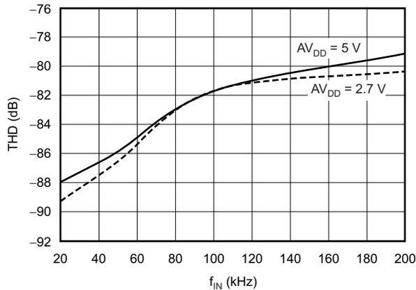
**Figure 22. TOTAL HARMONIC DISTORTION vs INPUT SIGNAL FREQUENCY**
