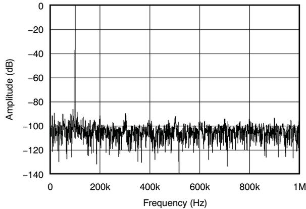
**Figure 16. FREQUENCY SPECTRUM (4096-Point FFT;  $f_{IN} = 100\text{ kHz}$ )**
