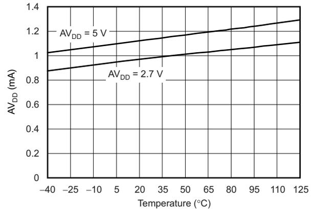
**Figure 29. ANALOG SUPPLY CURRENT vs TEMPERATURE (Auto-NAP Mode)**
