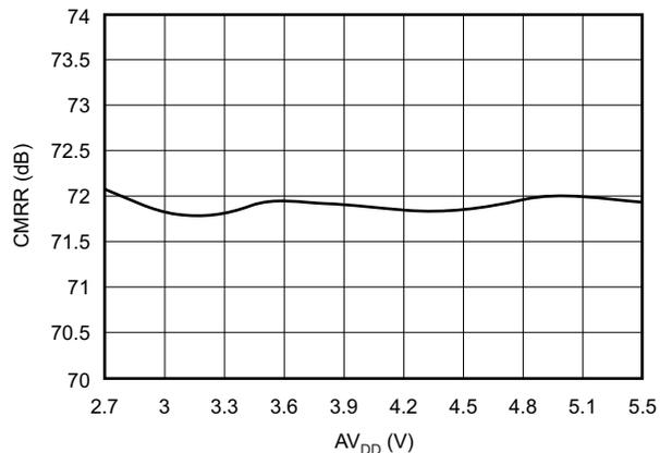
**Figure 14. COMMON-MODE REJECTION RATIO vs ANALOG SUPPLY VOLTAGE**
