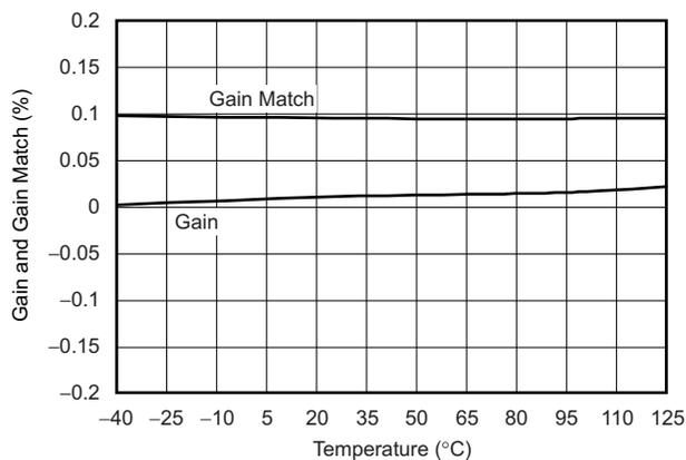
**Figure 13. GAIN ERROR AND GAIN MATCH vs TEMPERATURE**
