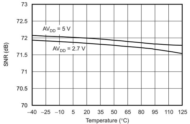
**Figure 21. SIGNAL-TO-NOISE RATIO vs TEMPERATURE**
