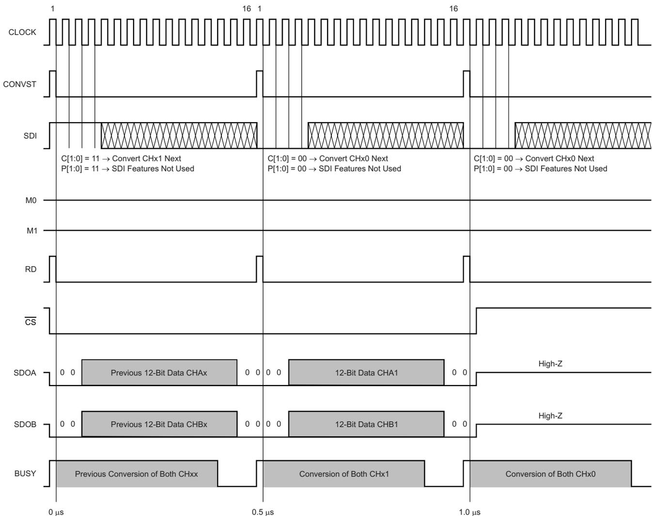
**Figure 33. Mode I Timing Diagram (M0 = 0, M1 = 0)**
