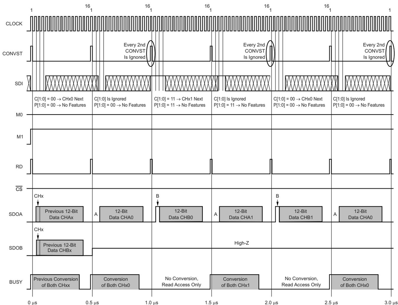
Figure 34. Mode II Timing Diagram ( $M0 = 0$ ,  $M1 = 1$ )
