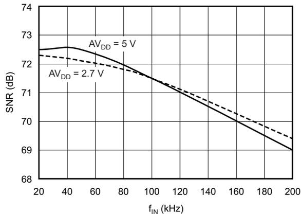
**Figure 20. SIGNAL-TO-NOISE RATIO vs INPUT SIGNAL FREQUENCY**
