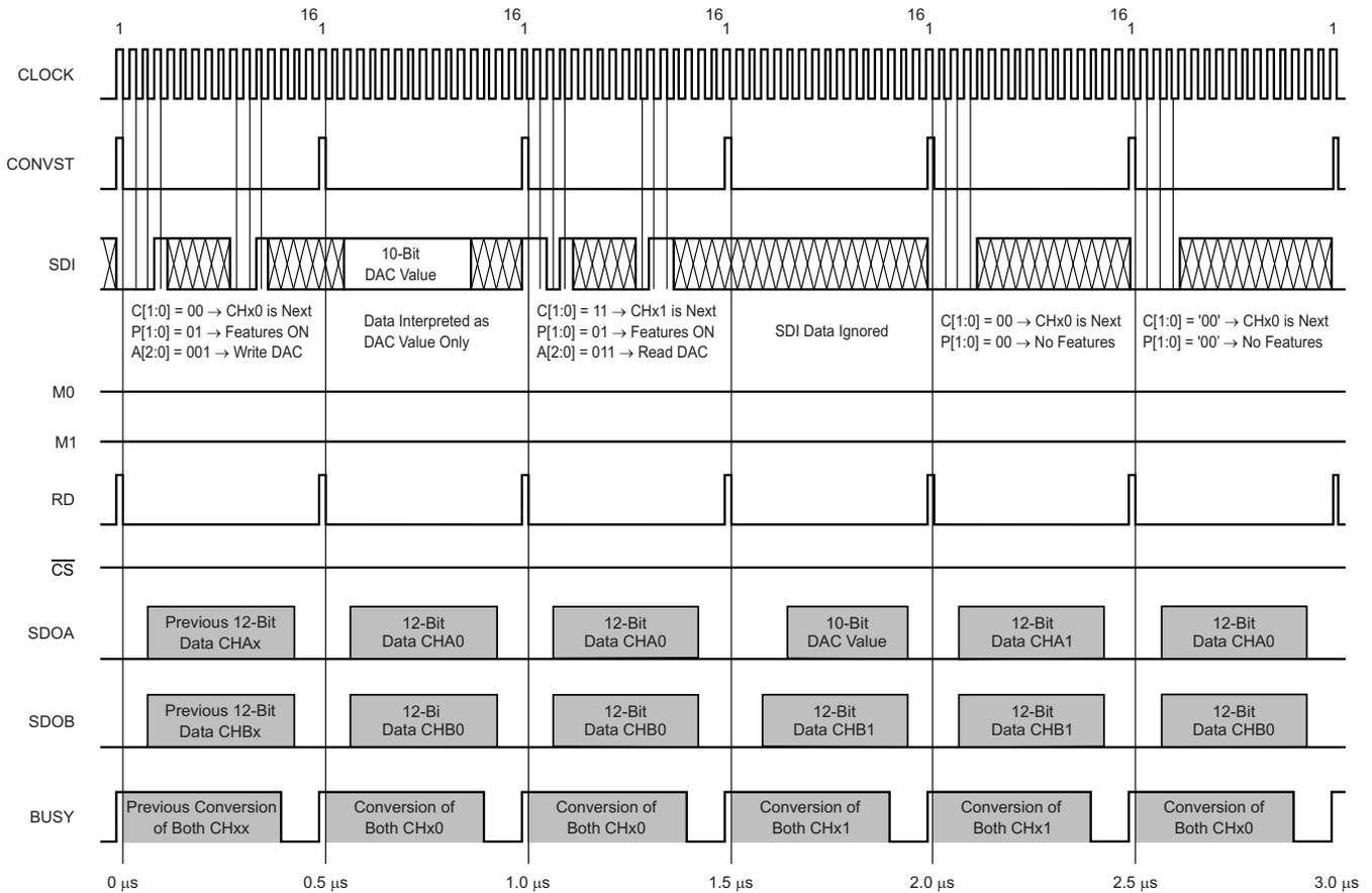
Figure 41. DAC Write and Read Access Timing Diagram
