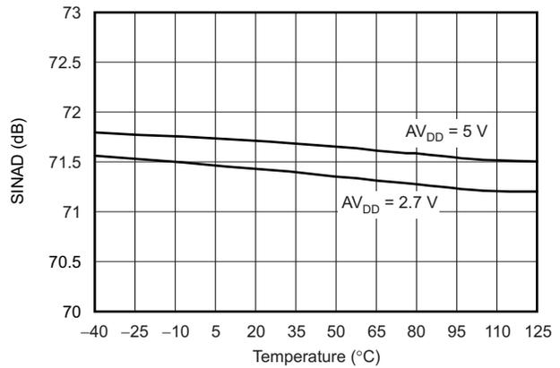
**Figure 19. SIGNAL-TO-NOISE RATIO AND DISTORTION vs TEMPERATURE**
