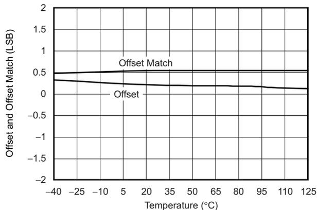
**Figure 11. OFFSET ERROR AND OFFSET MATCH vs TEMPERATURE**
