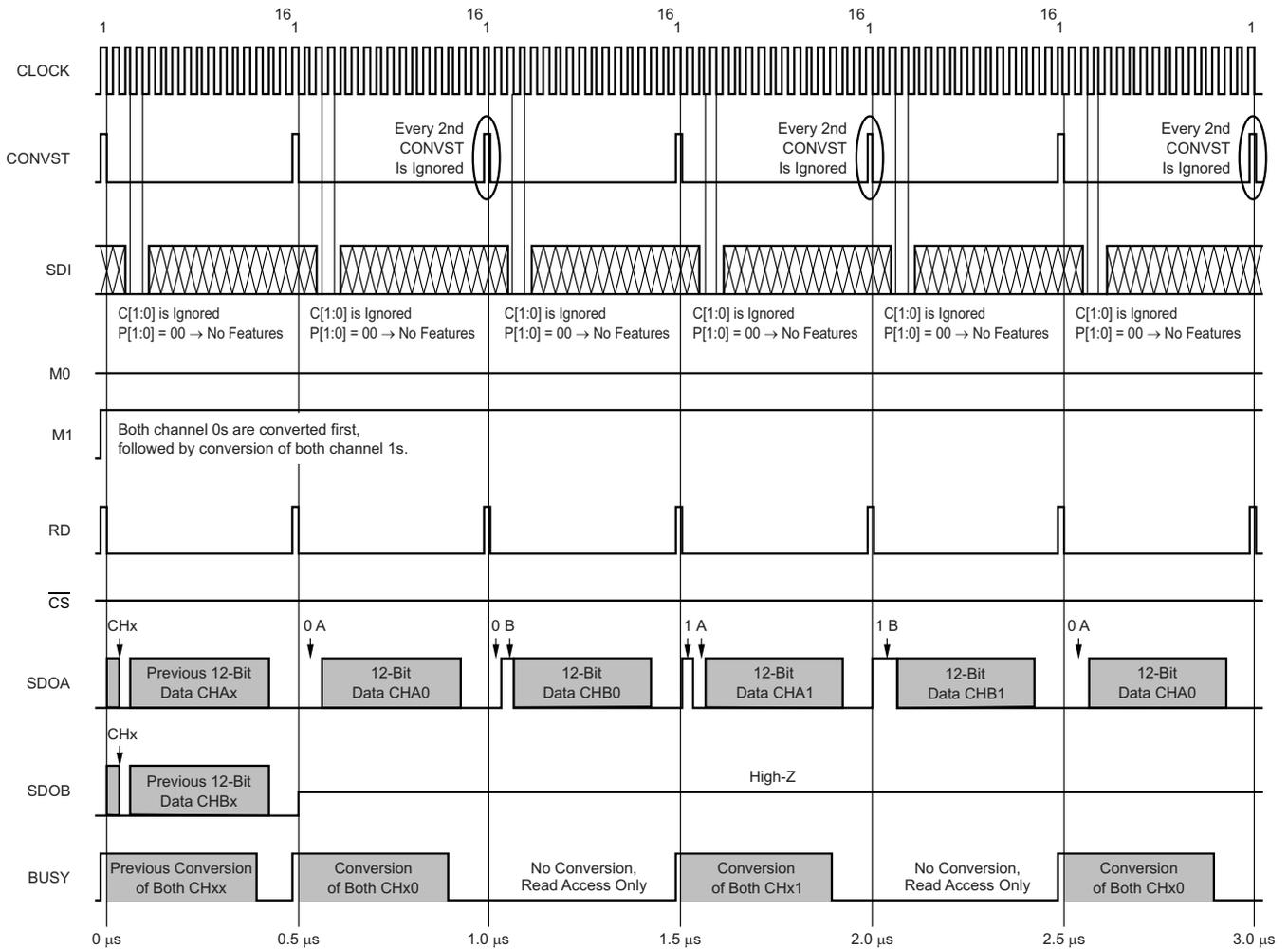
**Figure 36. Mode IV Timing Diagram (M0 = 1, M1 = 1)**
