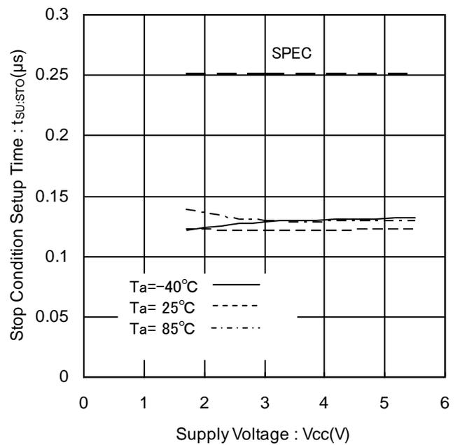
Figure 25. Stop Condition Setup Time vs Supply Voltage
