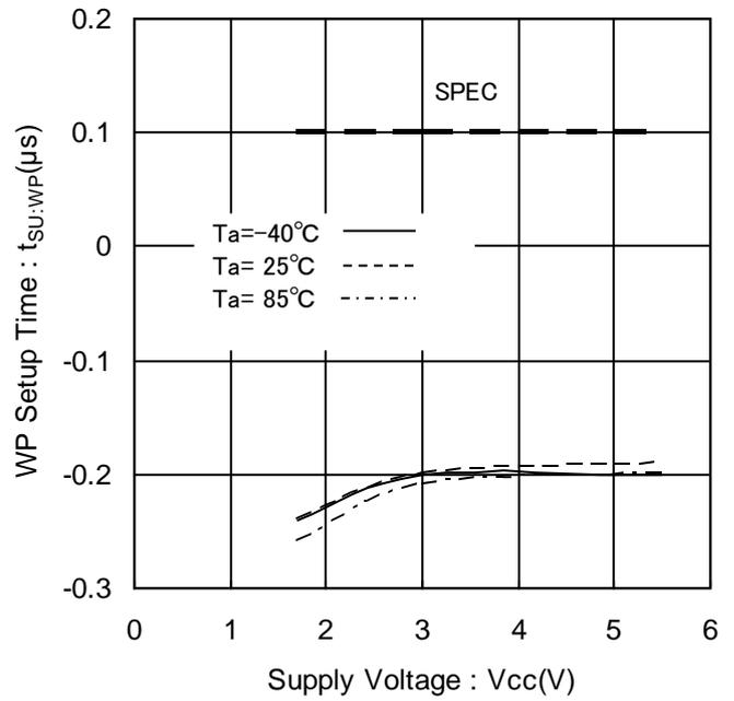
Figure 33. WP Setup Time vs Supply Voltage
