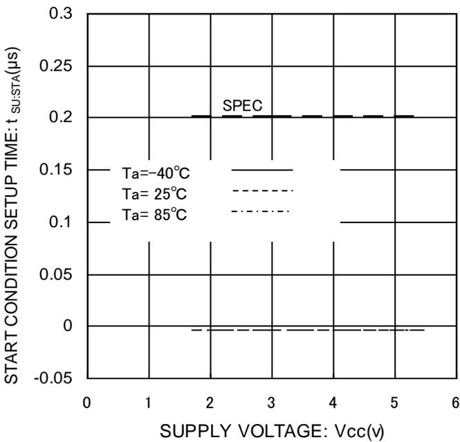
Figure 18. Start Condition Setup Time vs Supply Voltage
