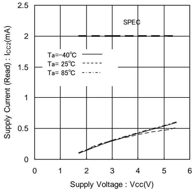
Figure 11. Supply Current (Read) vs Supply Voltage (f<sub>SCL</sub>=1MHz)
