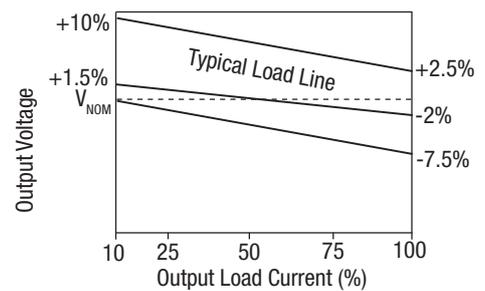
The voltage tolerance envelope shows typical load regulation characteristics for this product series. The tolerance envelope is the maximum output voltage variation due to changes in output loading.
