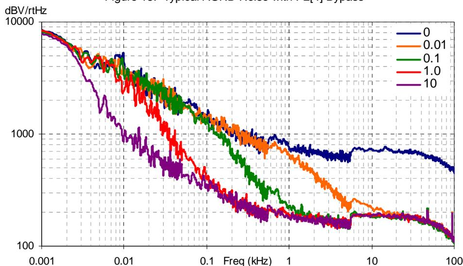
At low frequencies, the opamp noise is proportional to 1/f, power independent, and determined by device geometry. At high frequencies, increased power level reduces the noise spectrum level.
