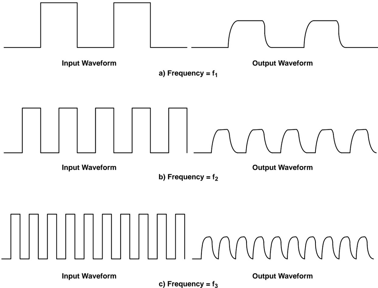
**Figure 9. Input and Output Waveforms of Filter**
