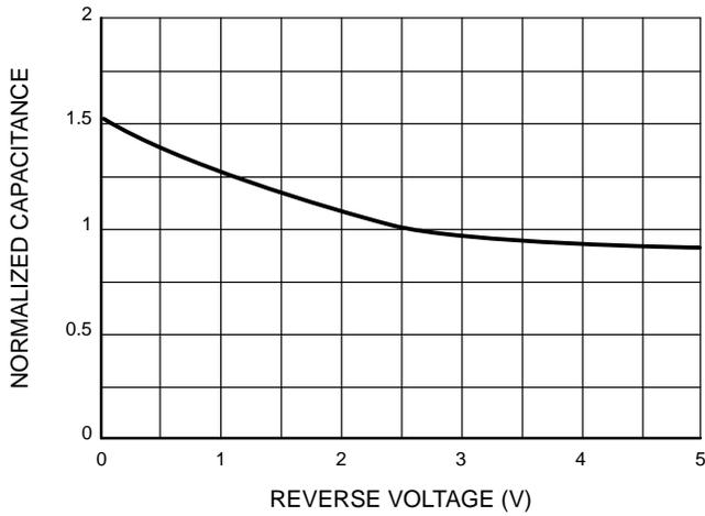
Figure 6. Typical Capacitance vs. Reverse Biased Voltage
