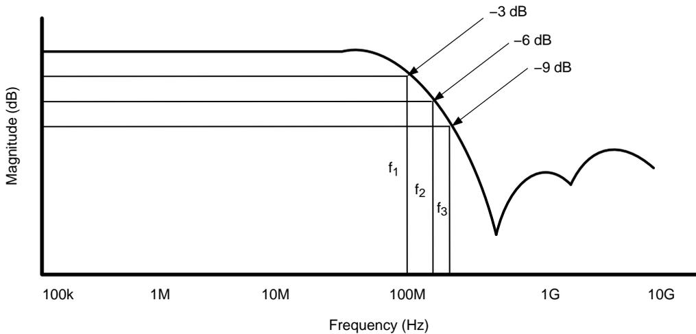
**Figure 8. Filter Bandwidth**
