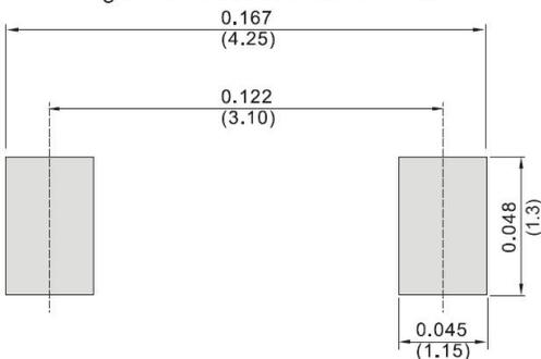
**Mechanical Dimensions SOD-123FL(Inches/Millimeters)**
