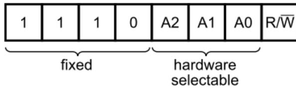
Figure 4: Device address
