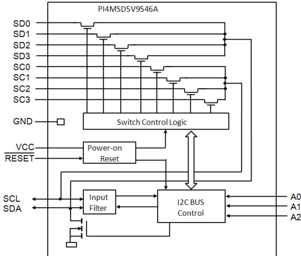
Figure 1: Block Diagram
